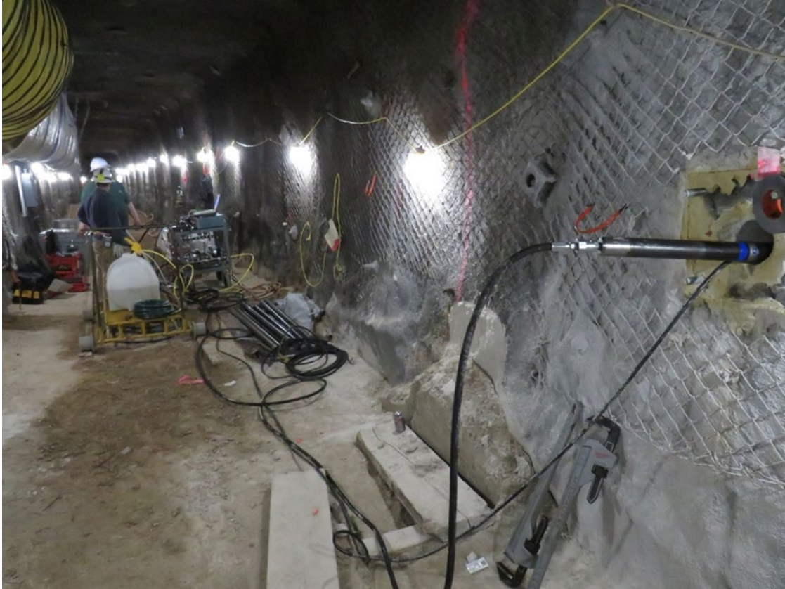
Figure 21. Photograph of the Hydrofracture system being run in GI-3.
