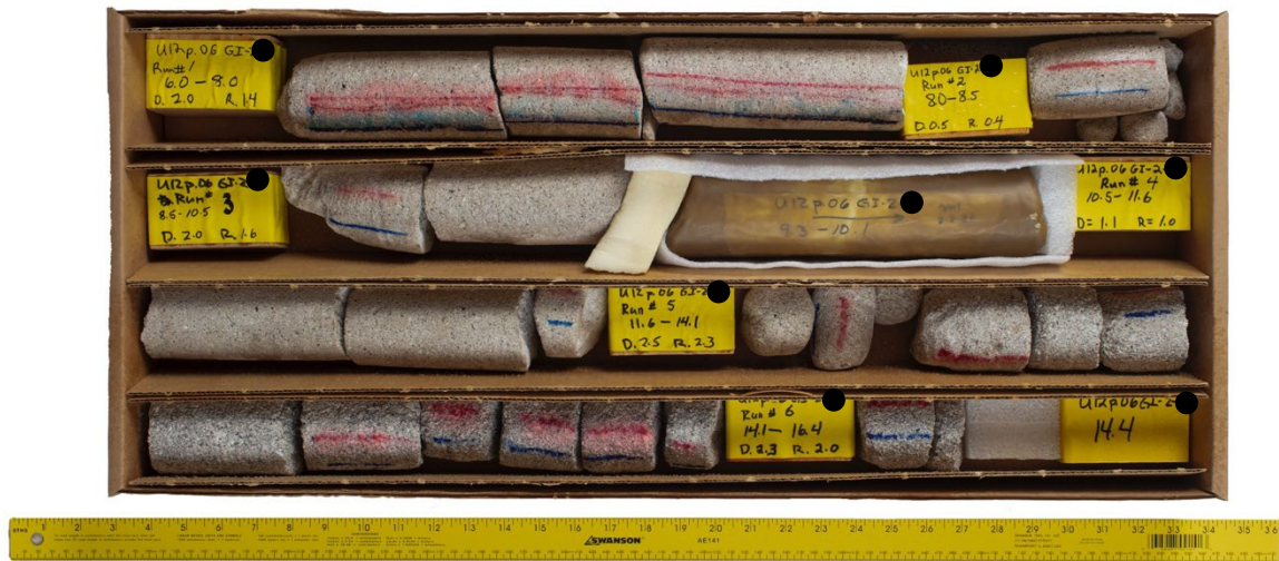
Figure 15. Example of the high-resolution photographs taken for the PE1 core in the USGS Core Library. This example is from the GI-2 borehole under dry conditions. Some samples are coated in wax to preserve water content.
