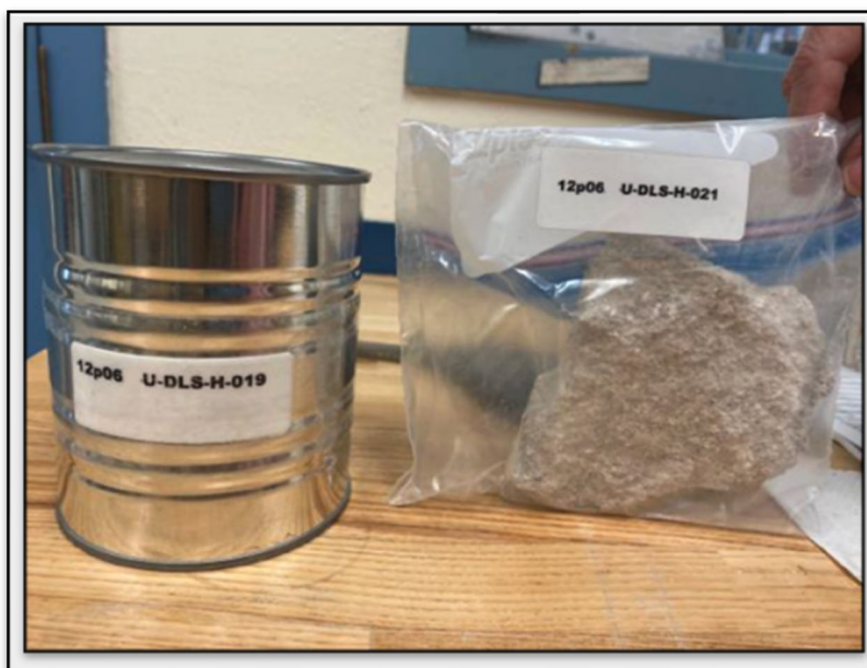
Figure 22. Photograph of two geologic grab samples from the 1490 drift. Leftmost sample is preserved, and rightmost sample is bagged.
