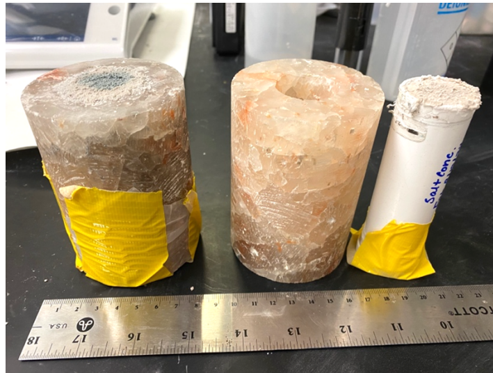
Figure 7: Types of salt core and salt concrete samples sent to GRS in FY24 (in-situ cured left, ex-situ cured right).
