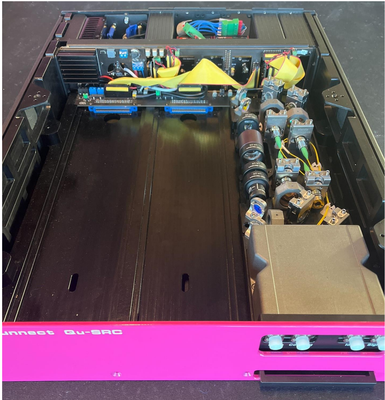
Figure 8: The photo of Qu-Source with inputs for the pump lasers and outputs for the entangled photons on the front. This unit comes with all the electronics needed in the back.
