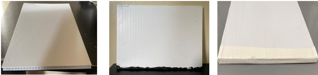
Figure 5. Three stages of the edge seal preparation – from the left: (i) Cleaning, and sanding the board edge, (ii) Butyl rubber tape is installed as a primary seal, and (iii) Vycor Pro tape is used as a secondary finish seal.
