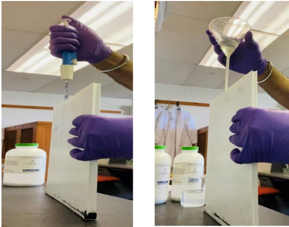
Figure 6. Extruded channel panel is filled with PCM using a pipette and a lab funnel.
