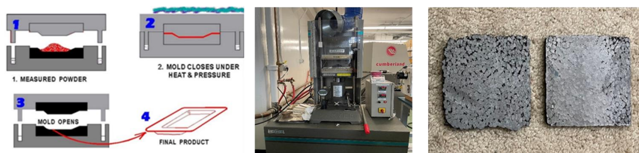
Figure 1. Process for compression molding (left). Carver, compression molder used during the project (center). Thermally conductive plastic molds, developed during the project (right).
