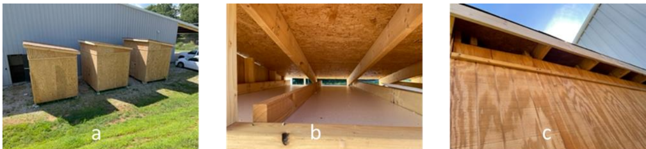
Figure 11. Installation of three test huts (a). Ventilated attic with shown attic insulation on bottom (b). Attic ventilation (c).
