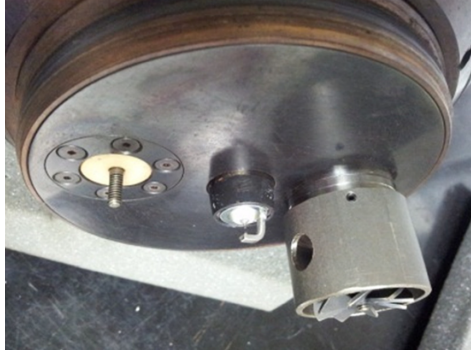
FIGURE 1. Interior of Combustion Vessel with Shrouded Fan to Generate Flow across the Spark Plug Gap
