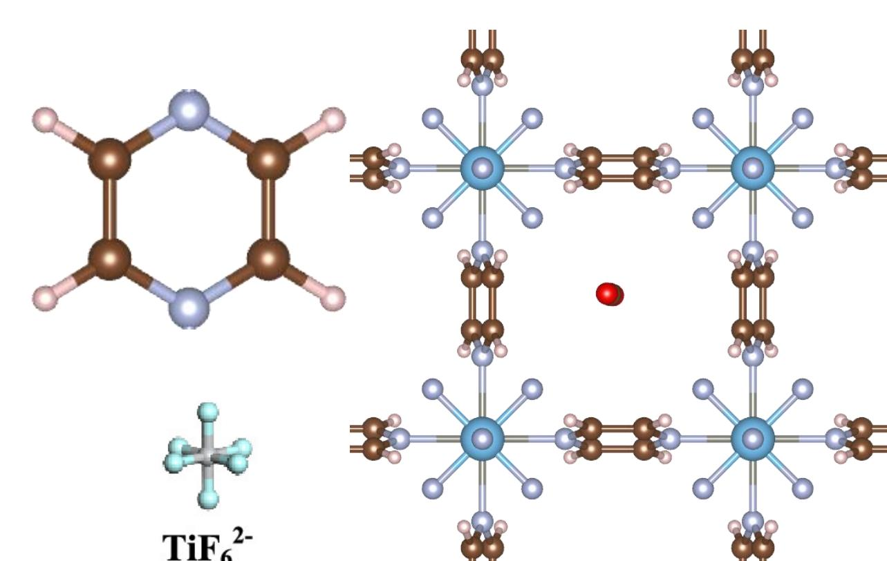
The optimal linker (pyrazine) and the CO<sub>2</sub> adsorption site in one of the best performing MOFs, TIFSIX-3-Zn.
