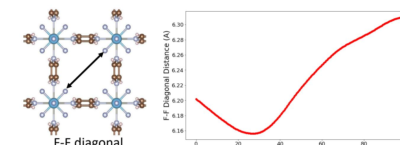
The fluorine-fluorine diagonal distance in the pores of TIFSIX\_3\_Zn as a function of time in an AIMD run.
