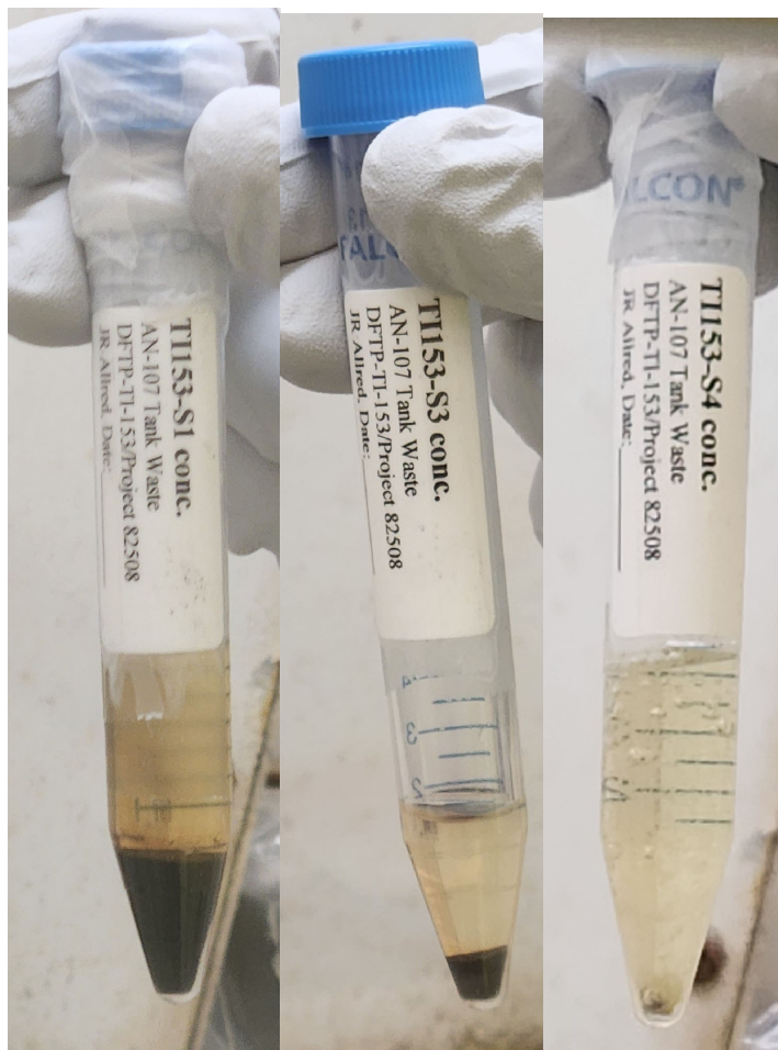
Figure 3.6. Concentrated solids in fume hood after centrifuging.
