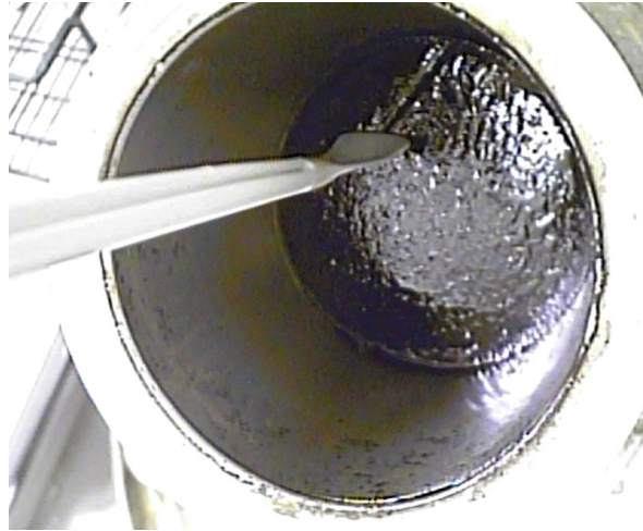
Figure 3.7. Solids being collected from DEF membrane in the Shielded Analytical Laboratory.
