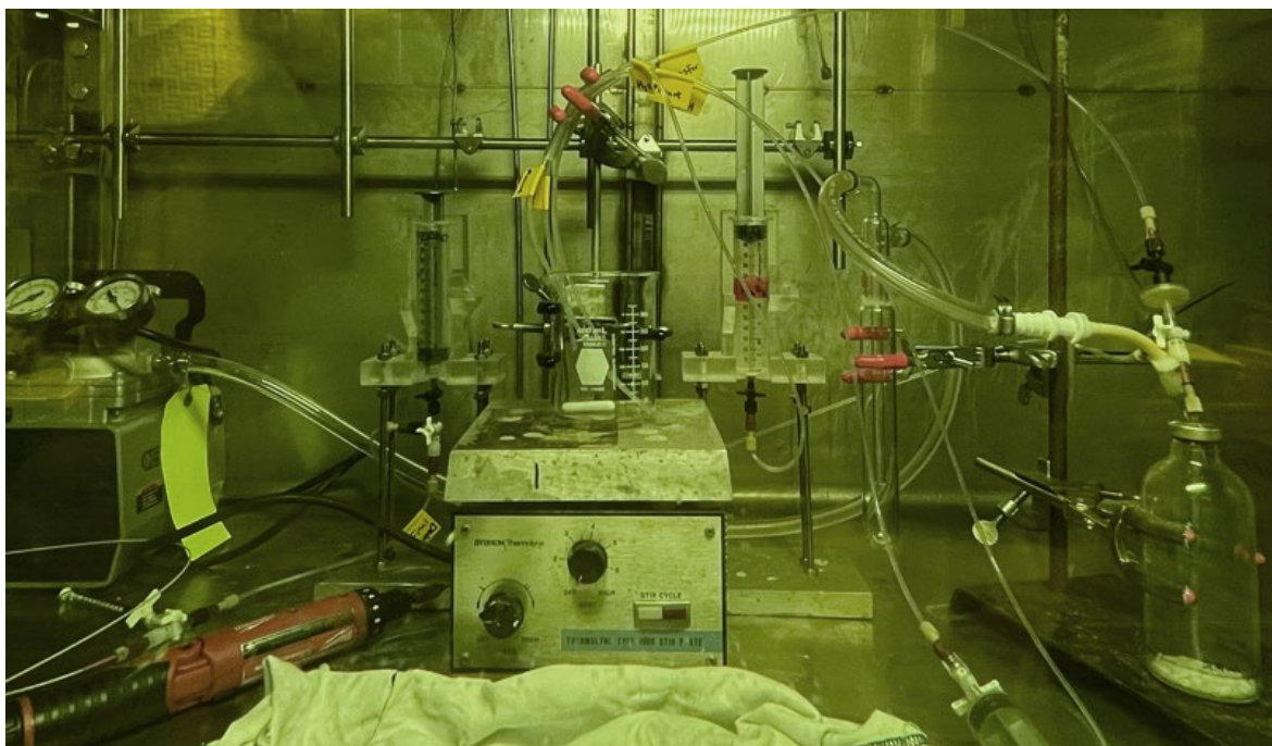
Figure 7 – The processing apparatus for dissolution of Mo disks and conversion to \text{K}_2\text{MoO}_4 , shown here in the hot cell.
