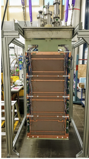
Figure 5. Module 0 before being placed in a cryostat for commissioning at the University of Bern. Visible is the back of the anode plane (pixelated charge readout) with the light readouts placed on the sides. At the top of the module one finds the vacuum insulation and feed-throughs.
