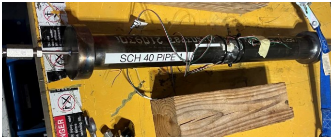
Figure 6. Pressure burst test setup for SCH-40 Pipe 1.
