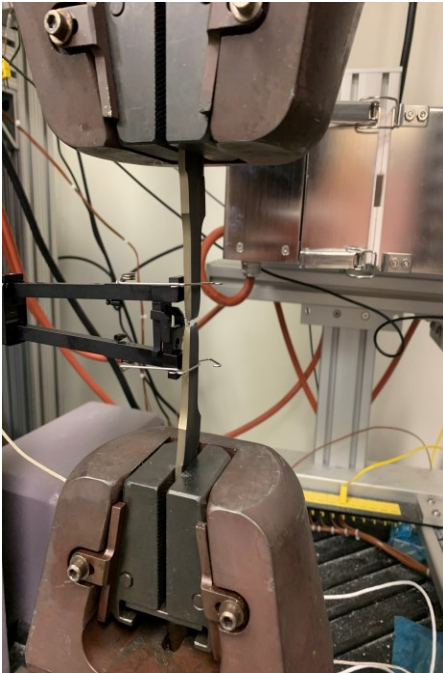
Figure 4. Tensile specimen fixture.
