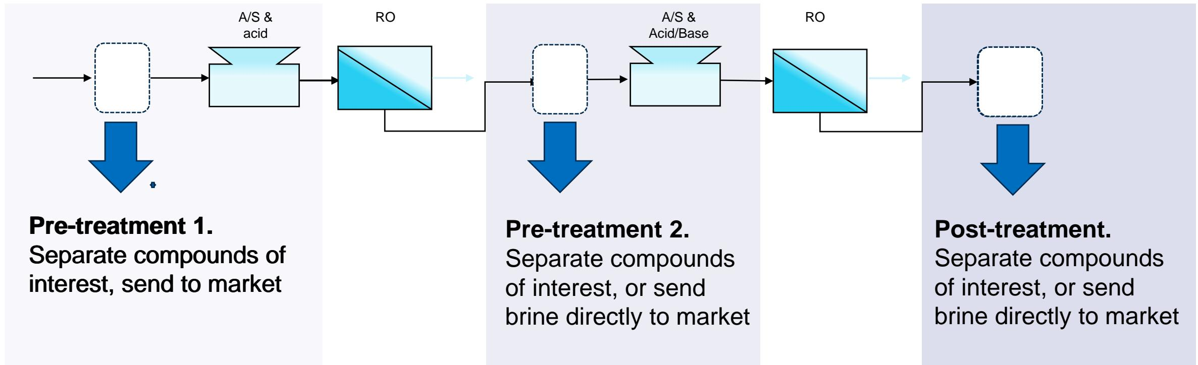
**Valorization processes:** Chemical precipitation, thermal precipitation, selective separation (ion exchange, nanofiltration, and selective electrodialysis), membrane or diaphragm electrolyzers, bipolar membrane electrodialysis
