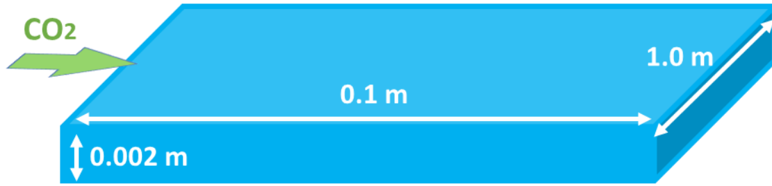
Fig.6 Sketch of the setup for the Buckley-Leverett problem.
