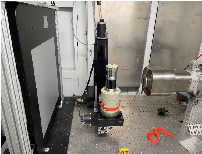
Figure 3: Experimental Setup with Deben CT5000RT Mounted in CT Booth
