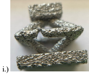
Figure 2: As built defect lattices for conditions: a) Standard b) Missing Strut, c) Slant 50%, d) Wave 50%, e) Thin 25%, f) Rapid Thin 50%, g) Long Thin 25%, h) Kink+Diameter 50%, i) Shifted Kink 75%
