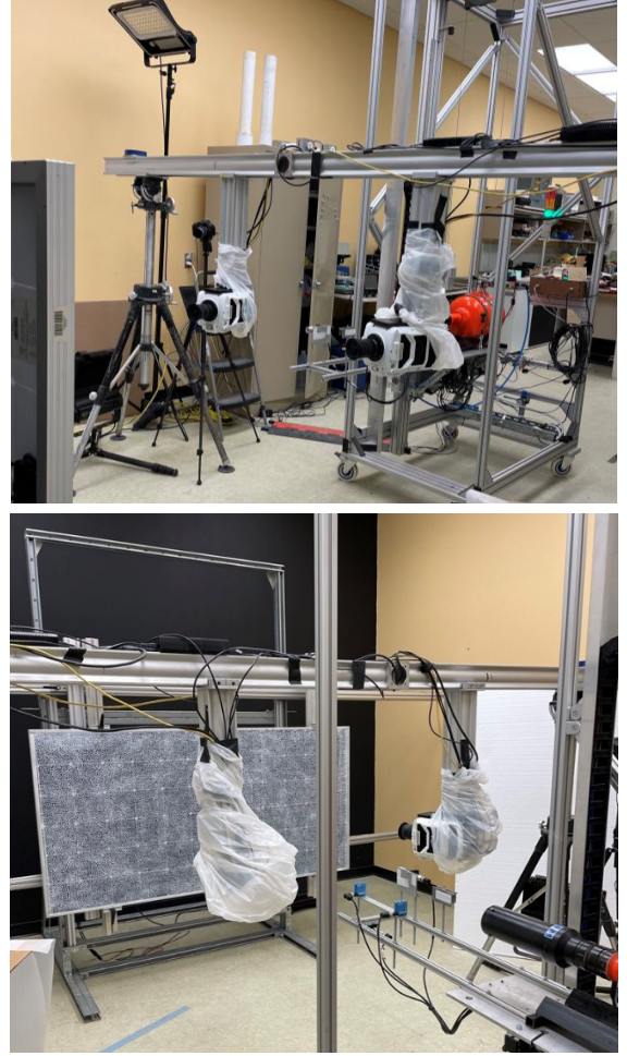
Fig. 1. Hail testing setup with high speed video acquisition equipment.
