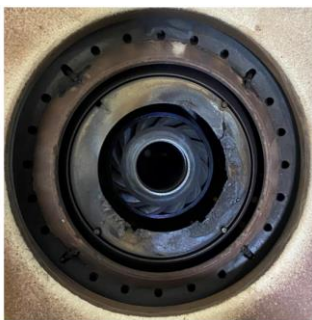
FIGURE 15. Image of fuel nozzle and guide swirler condition post-test. Minor distress is noted on the fuel nozzle endcap, while no distress is evident on the internal fuel/air mixer. The endcap distress is believed to have occurred during a short transient when water was reduced significantly while operating on 100% hydrogen.
