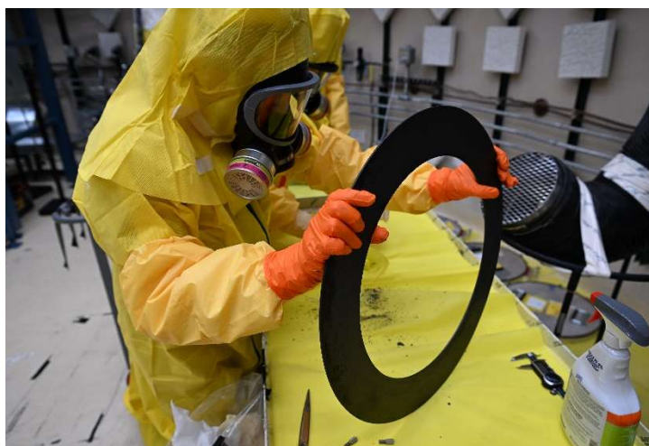
A 21/15 HEU Pancake plate being cleaned.
