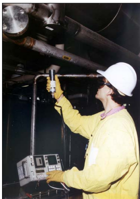
Figure VIII.4. a). A collimated NaI detector (radial response described by Figure VIII.3) measures the gamma-ray spectrum of holdup in the pipe at the location marked by the white bar-coded label. This vertical pipe appears as a narrow line in the detector's relatively wide field of view at this measurement distance. The finite-source effect on the specific mass for the line deposit is small in this case. b). The same detector is positioned at the same measurement distance from a second bar-coded measurement location on a horizontal duct whose diameter is four times that of the vertical pipe in a). Proximity of the neighboring overhead equipment may prevent use of a larger measurement distance without including additional deposits in the field of view. The horizontal duct appears as a broad line in the detector's somewhat wider field of view at this measurement distance. The finite-source effect on the specific mass for the line source is much larger in this case.
