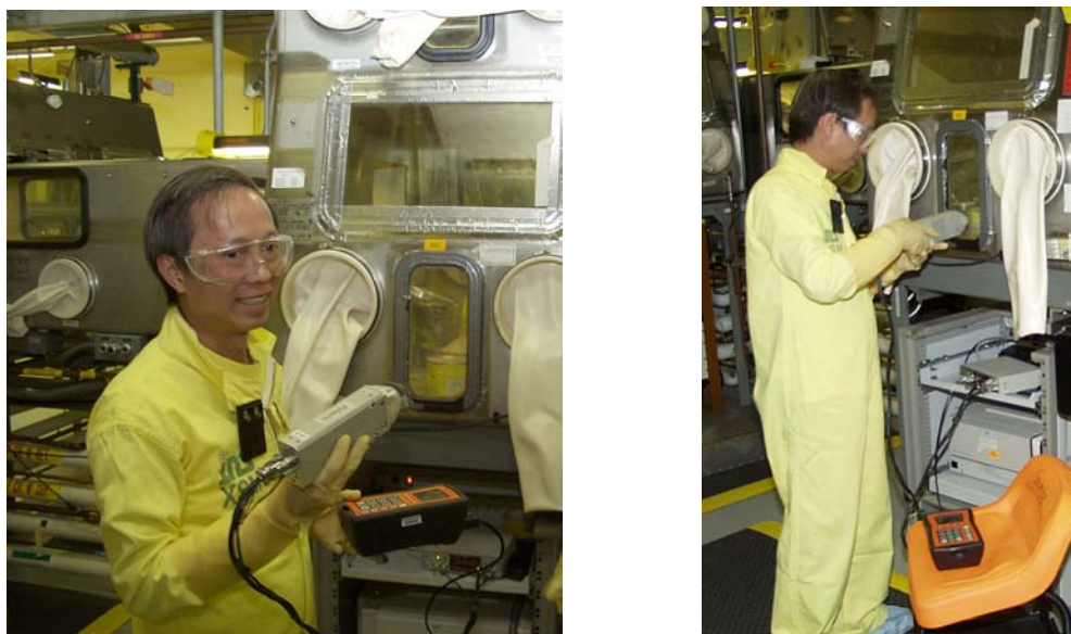
Figure VII.11. The Peltier-cooled portable CdTe detector is shown in use for portable isotopics measurements of plutonium in a process glove box.
