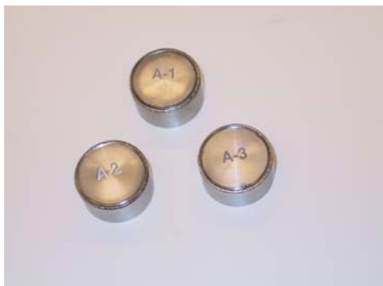
Figure VI.3. One of the five sets of encapsulated plutonium metal foil standards includes three thicknesses (0.6, 1.3 and 2.5 g Pu/cm 2 ). Each low-burnup (93.9% 239 Pu) foil has a 2-cm diameter.
