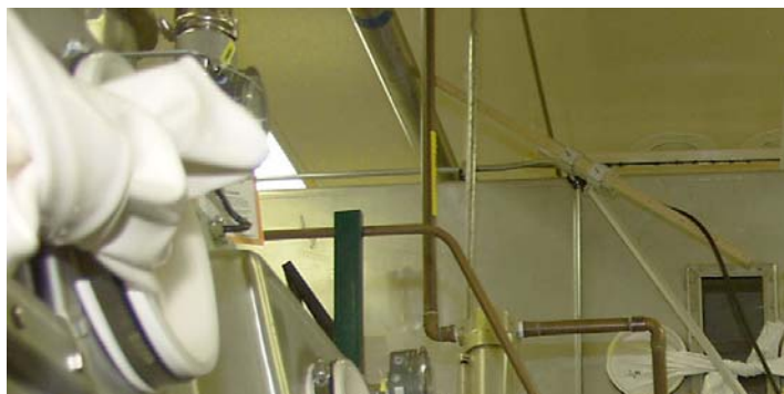
Figure VII.8. The compact NaI detector (see Fig. VII.6) is shown during measurements of plutonium deposits in overhead ducts. The detector is mounted on a telescoping pole. The bottom-frame exploded view from the middle frame shows a wooden meter stick used as a positioning standoff from the duct.
