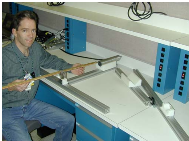
Figure IX.1. A mechanical positioning device is shown in use for calibrating the 2.5-cm by 5.0-cm compact NaI detector to measure LEU. The calibration standard is mounted on the detector axis at r_0 = 40 cm. An additional device shown at the right (nearly fully collapsed for storage) illustrates the variable position of the calibration standard, detector distance, and relative angle between source and detector axes allowed by this simple device.
