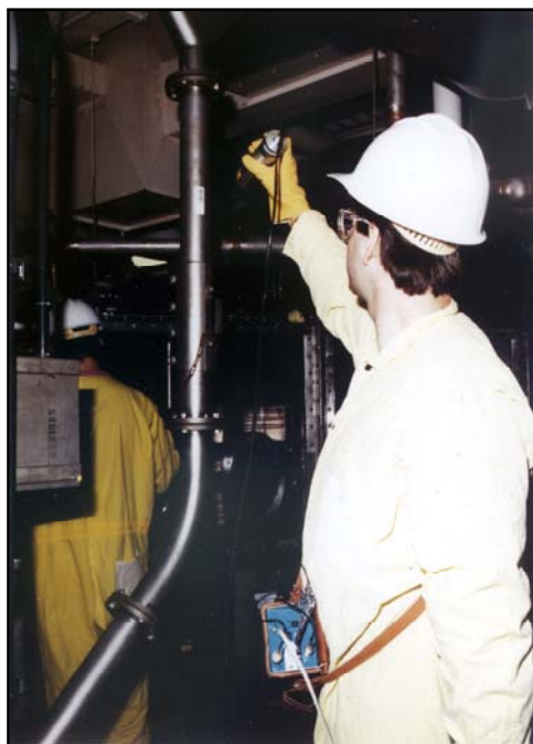
Figure VIII.4. a). A collimated NaI detector (radial response described by Figure VIII.3) measures the gamma-ray spectrum of holdup in the pipe at the location marked by the white bar-coded label. This vertical pipe appears as a narrow line in the detector's relatively wide field of view at this measurement distance. The finite-source effect on the specific mass for the line deposit is small in this case. b). The same detector is positioned at the same measurement distance from a second bar-coded measurement location on a horizontal duct whose diameter is four times that of the vertical pipe in a). Proximity of the neighboring overhead equipment may prevent use of a larger measurement distance without including additional deposits in the field of view. The horizontal duct appears as a broad line in the detector's somewhat wider field of view at this measurement distance. The finite-source effect on the specific mass for the line source is much larger in this case.
