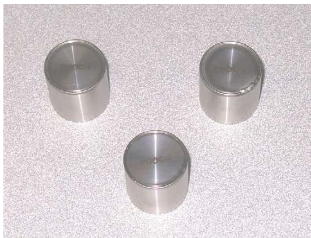
Figure VI.4. One of the five sets of encapsulated plutonium oxide standards includes three thicknesses (0.4, 0.9 and 1.8 g Pu/cm 2 ). The oxide in each low-burnup (94.0% 239 Pu) standard is confined to a cylinder that is 2.7 cm in diameter.
