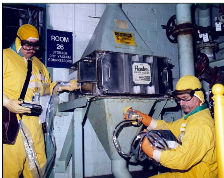
Figure VII.7. Top: Portable measurements of ^{235}\text{U} deposits in a process filter system are performed with a portable Ge detector weighing ~10 kg with its tungsten collimator-shield. Bottom: CZT and NaI also in use for measurements of process filters weigh ~1 kg each with their respective tungsten and lead shields.
