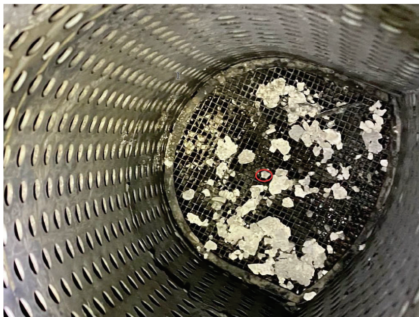
Figure 3-11. Similar Solids from Prior Caustic Dissolution of Aluminum Cladding – Test 6 of SRNL-STI-2020-00264. 7
