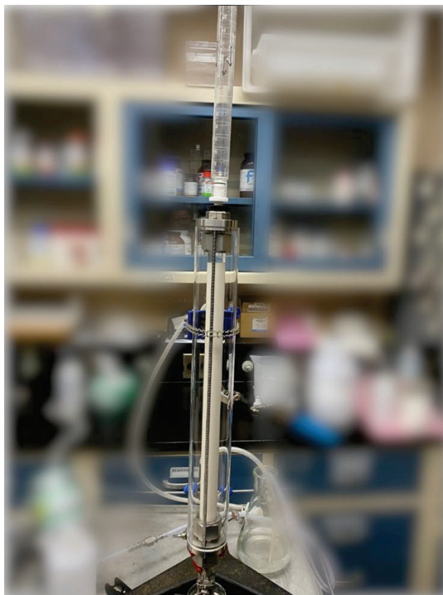
Figure 3-19. Final Elutriated, Settled, and Packed Reillex Column Used for Mark-18A Water Evaluations and Cold Simulant Testing.
