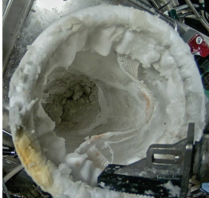
Figure 3-17. Contents of FLT-315 after cold run filtration
