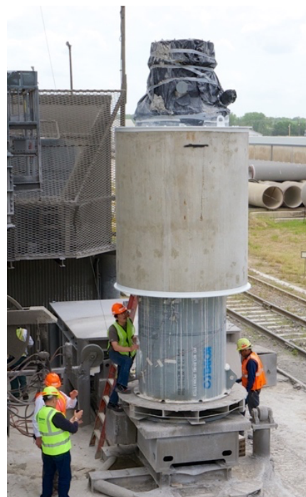
Figure 6 Hydrogen storage vessel cost of ORNL GEN II SCCV technology [18]. The photo shows a SCCV is being manufactured in a vessel company in Texas.
