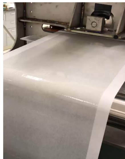
Figure 10. (a) Close-up of the dual slot die. (b) Dual slot die in operation.
