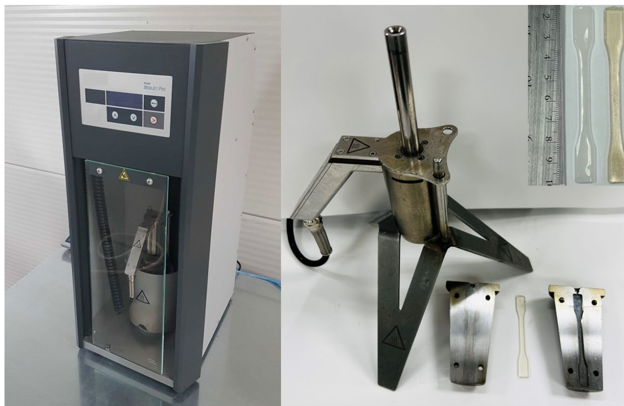
Figure 2. The injection molder, cylinder, mold, and Type 3 dog bone specimen used in this study. In the upper right-hand side is a sample of K705 (left) and PVDF-CTFE (right).
