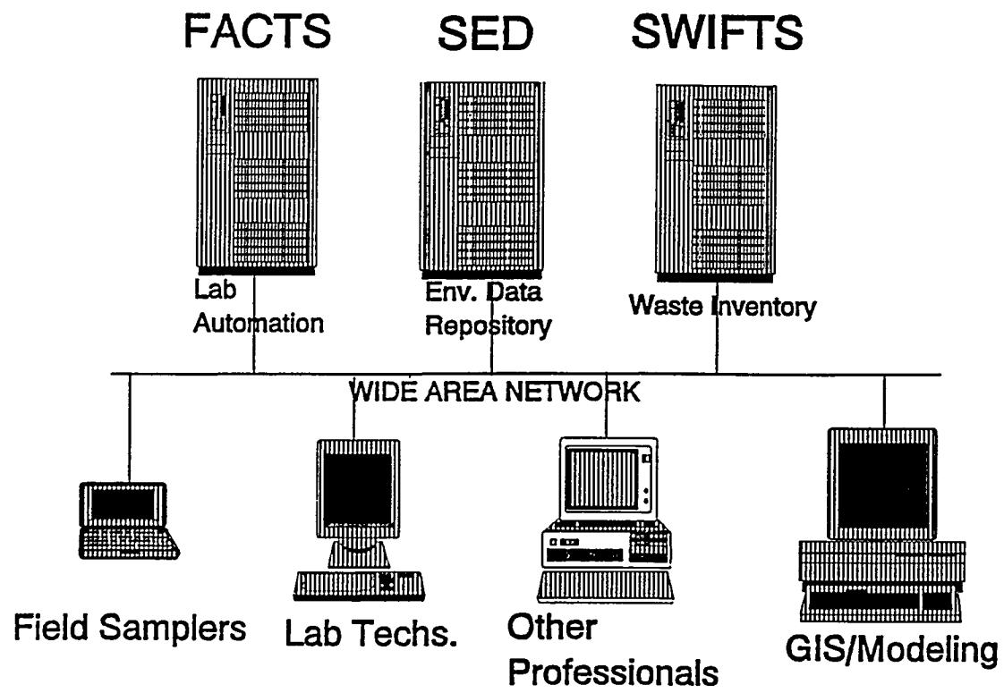
Figure 1 Schematic of Environmental Systems
