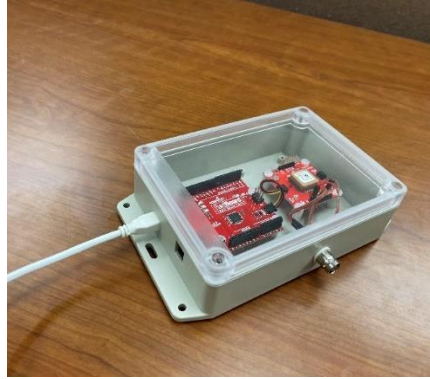
Figure 152. GPS Pulse Generator assembled into polycarbonate enclosure for 3 rd scope location.
