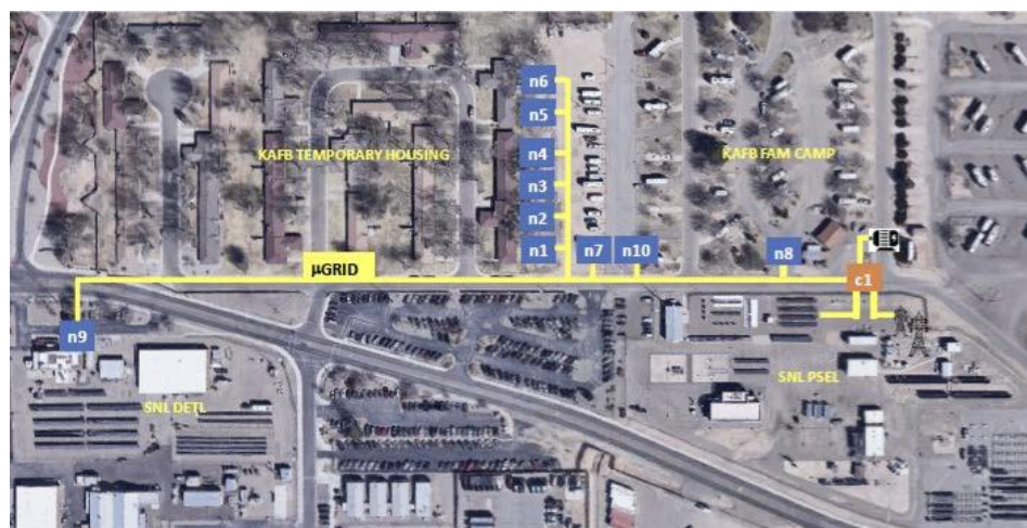
Figure 146. KAFB DC microgrid serving housing, utility, and DETL sites.
