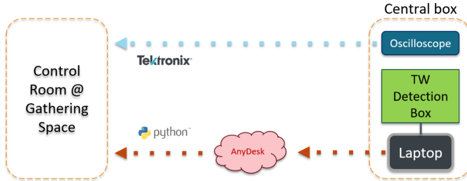
Figure 181. Data flow in the presented testing methodology, assuming that the DSP box is located at the Central Box.
