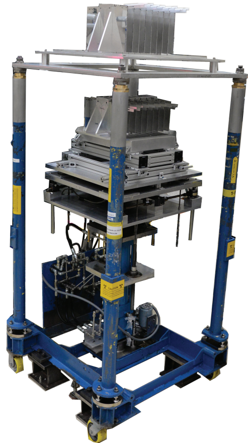
Fig. 3. 8 \times 1 configuration on the Planet critical assembly machine. Here the platen is in the fully lowered position.
