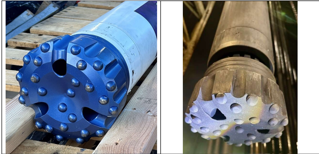
Figure 19. Percussive hammer (DTH) before (at left) and after drilling 40ft (at right).
