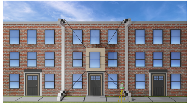
Figure 1. Conceptual view of a cable-driven parallel robot for retrofitting a residential building using overclad panels in a densely populated urban area.
