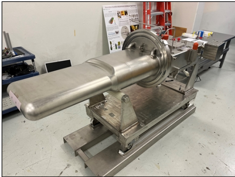
Figure 4: First production 2 MW target at SNS.
