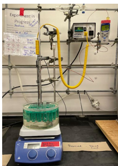
Fig. 5.4. Water bath reactor with temperature controller for local optimal aldol-condensation reactions conditions at NCSU.
