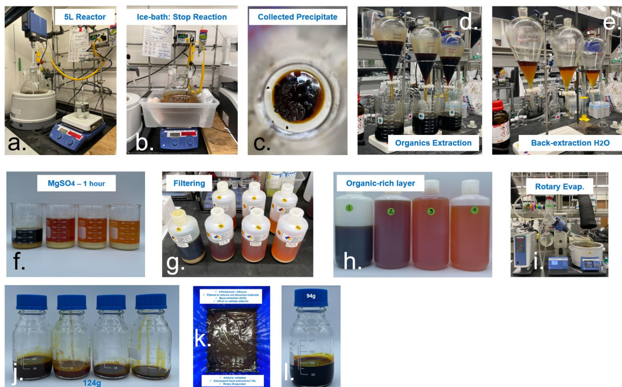
Fig. 5.14. Big-scale aldol-condensation reaction experiments: (a) 5L reactor with overhead stirrer. (b) Ice-bath to stop the reaction. (c) Precipitated sludge left after neutralization of the reaction volume. (d) Organic liquid-liquid extraction using 2-pentanone. (e) Back extraction using DI water. (f) Water removal from organic layer collected during extractions 1 to 4 using \text{MgSO}_4 . (g) Collected organic layers before \text{MgSO}_4 filtration. (h) Filtrated organic layer from extractions 1 to 4. (i) Rotary evaporator for 2-pentanone removal. (j) Aldol-condensation products collected after 2-pentanone removal. (k) Collected precipitated sludge before 2-pentanone extraction. (l) Additional aldol-condensation products extracted from precipitated sludge.
