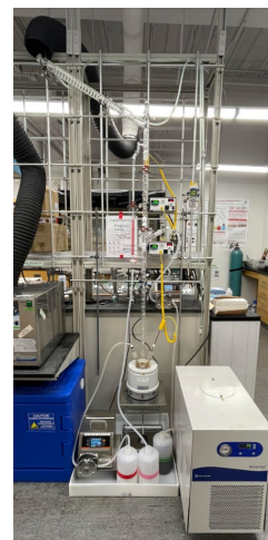
Fig. 7.5. (a) Vapor-liquid equilibrium for the binary system 1,4-dioxane/water and acetone/water from Aspen Plus™ and (b) In-house-built multi-stage continuous distillation system used at NCSU to distill co-solvents from the furan products solution produced at NREL.
