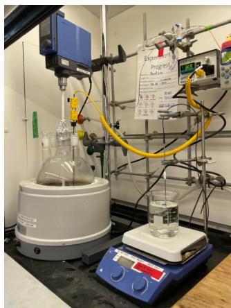
Fig. 7.10. Five-liter batch reactor for aldol-condensation at NCSU.
