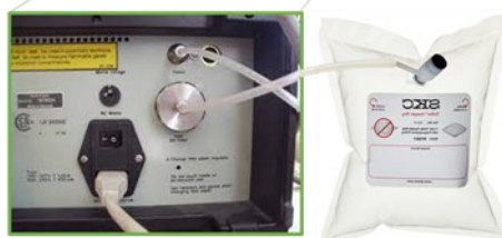
Figure B-1. Innova 1312 Photoacoustic Spectrometer and Sample Inlet
