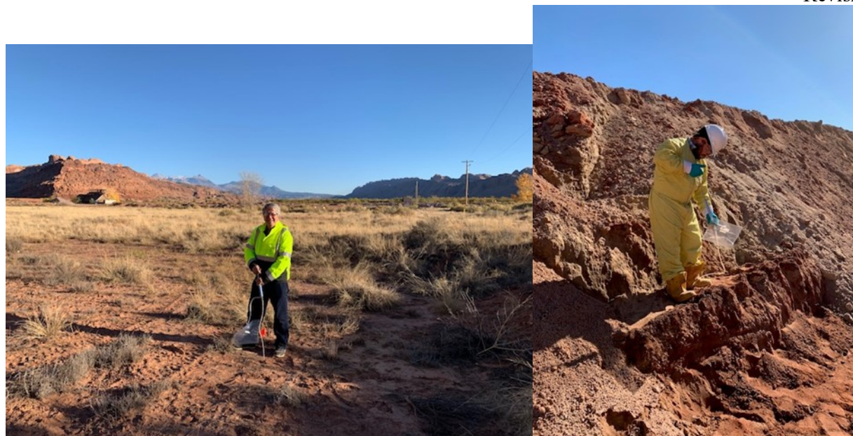
Figure 4-6. Collection of Soil Gas with Hand-Pump
