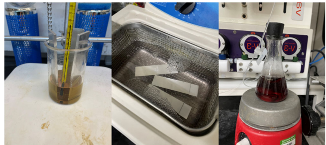
Figure 7: Left to Right, P 2 acid etching setup, ultrasonic Dirl-Lum 603 solution, and Ferric sulfate precursor solution.
