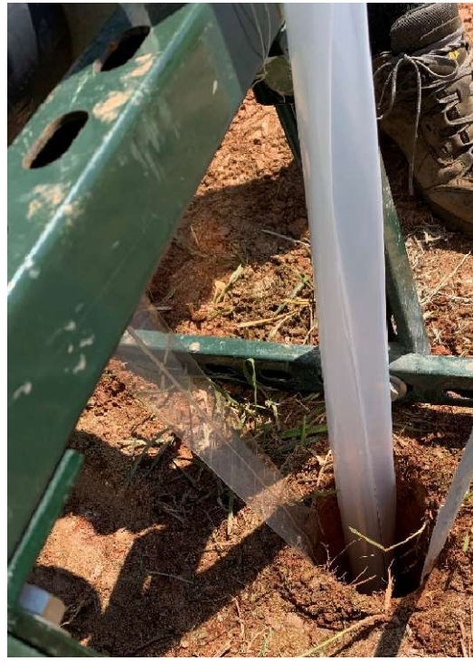
Figure 2.8: Installation of the polyethylene tubing in the borehole. a.) Strain ribbon (transparent) passing over a roller at the top of the borehole. Folded polyethylene sleeve is the white band at the top of the image; b.) Close up of the borehole with the transparent strain ribbon and the folded polyethylene sleeve.
