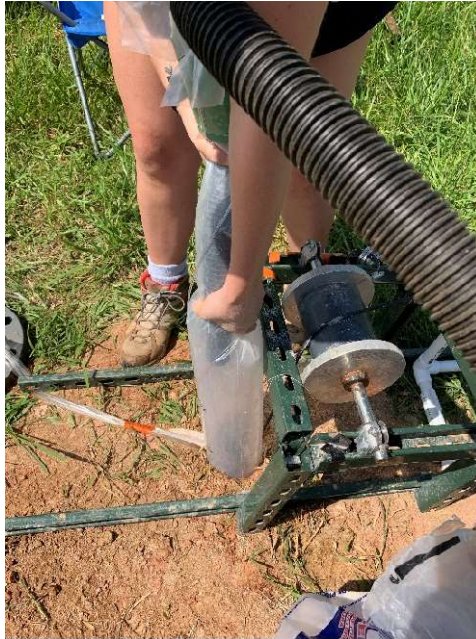
Figure 2.8c: Polyethylene sleeve is pressurized using a shop-vac pushing the strain ribbon onto the borehole wall.
