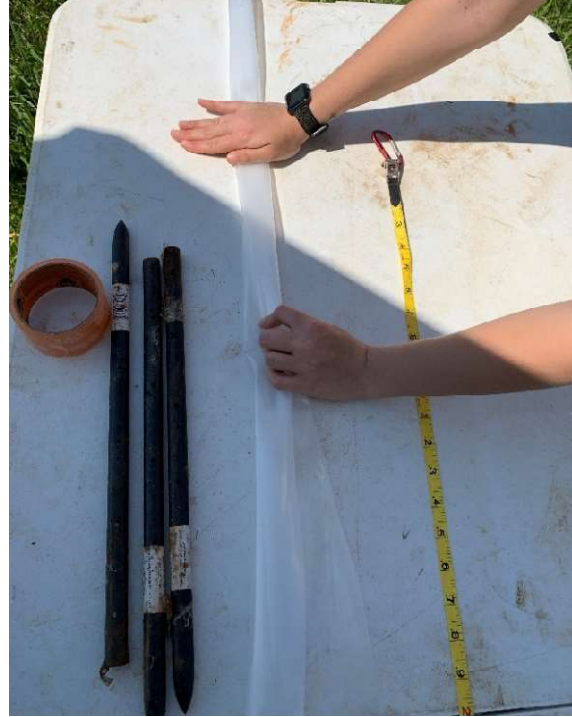
Figure 2.7: Polyethylene sleeve being prepared for installation in the borehole. a: Tubing meaning measured. b: Tubing being folded.
