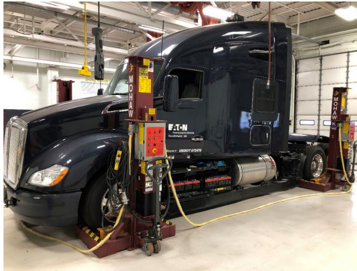
Figure 97: Kenworth T680 equipped with a (temporary) 48V Lead-Acid battery system
