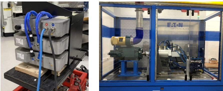
Figure 90: Battery system assembled into truck battery tray (left), and Integrated into Dyno (right)
