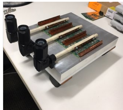
Figure 96: Mechanical Mockup of Inverter Components
