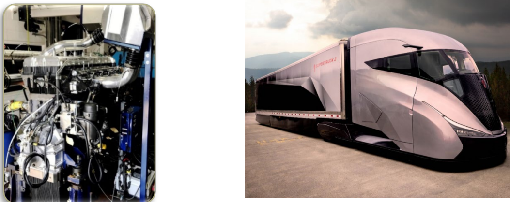
Figure 1: PACCAR MX SuperTruck II Engine (Left) and Kenworth SuperTruck II Vehicle (Right)
