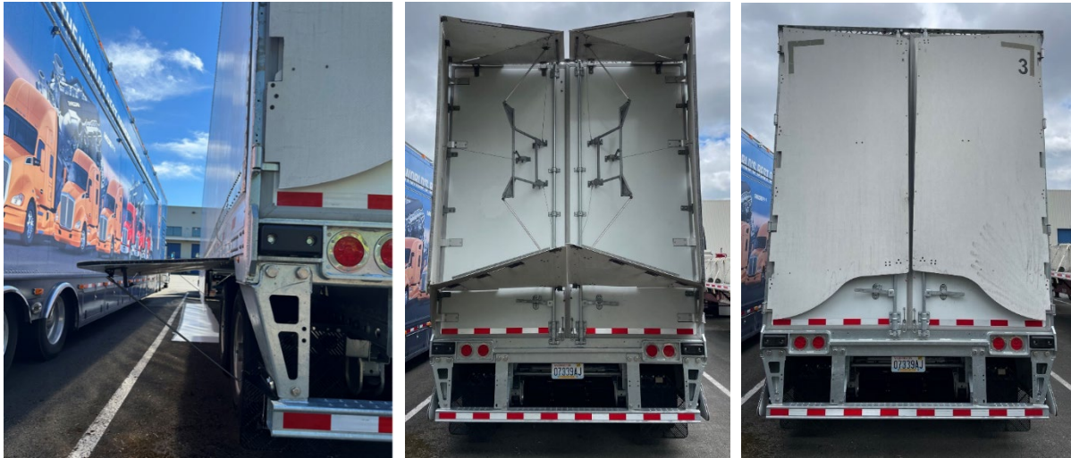
Figure 125: Trailer skirt prop rods, trailer boat tail deployed, and stored
