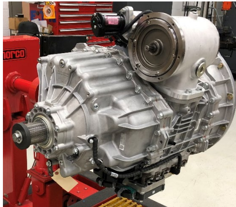
Figure 92: PTO Gearbox Test Fit on PACCAR 12 Speed Transmission
