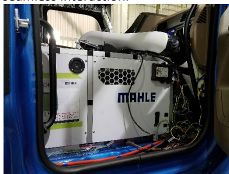
Figure 127: Heat Pump Assembly as fitted to Mule
