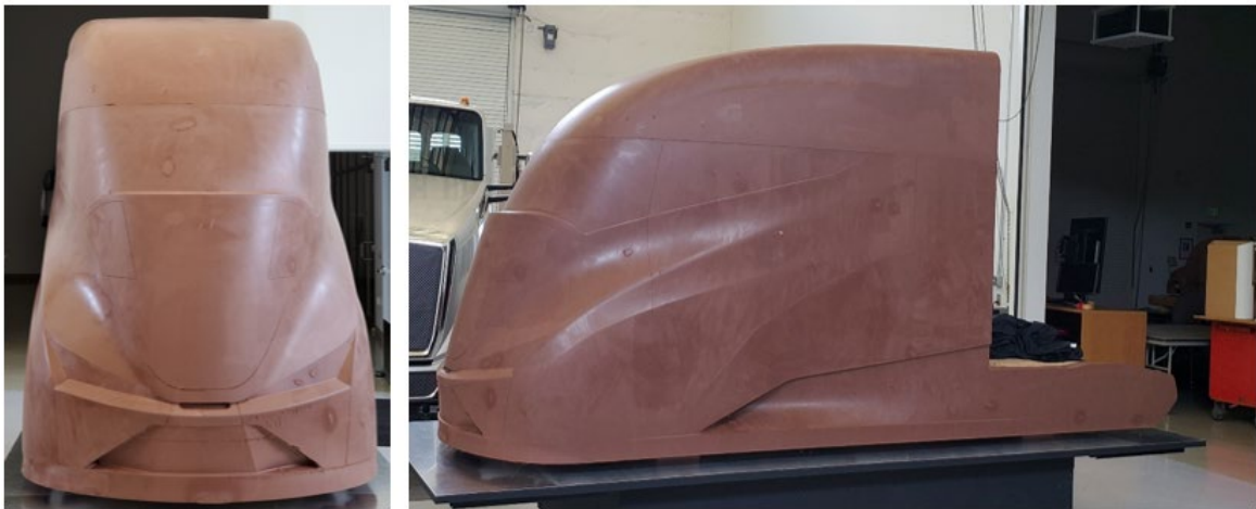
Figure 112: 50% Clay Model – Completed milling, roof assembled and ready for use by styling/design/engineering teams
