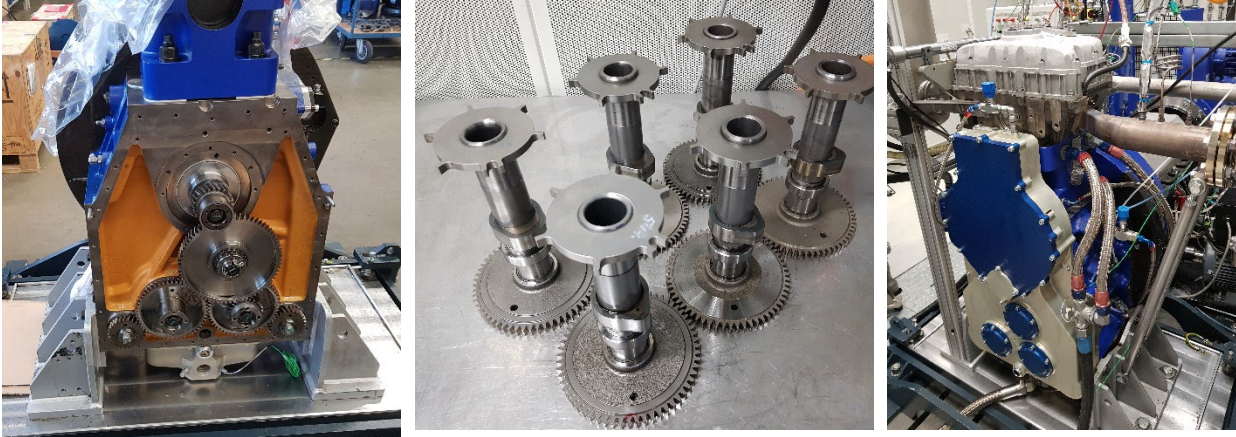
Figure 46: New long stroke SCE version of PACCAR MX-12 SuperTruck II engine (left), new Miller timing SCE camshafts (middle), and long stroke SCE test cell installation (right)
