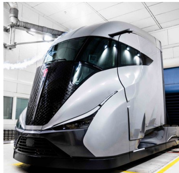
Figure 20: Kenworth SuperTruck II vehicle in the PACCAR Climatic Chassis Dynamometer
