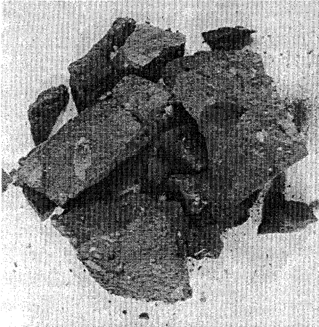
Figure 4: Macrograph of the starting material for this investigation. Note the light phase material which is very high interstitial content tantalum.
