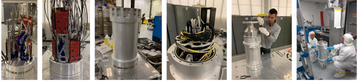
Figure 7. FIDDLE barrel in build after CMM metrology. Right. Barrel in Target Diagnostic “Factory” snout alignment calibration station.
