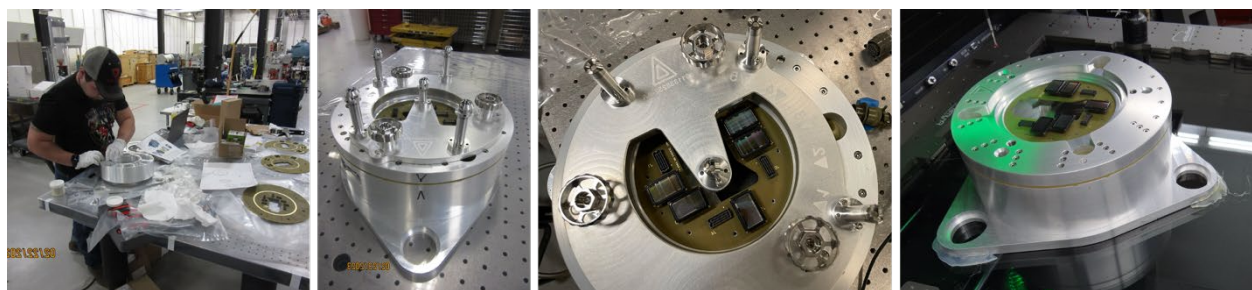
Figure 6. FIDDLE front end build photos Left to right: Front components in build by technician; After sensor installation with CMM metrology spheres side view and top view; In optical CMM lab for sensor location metrology.
