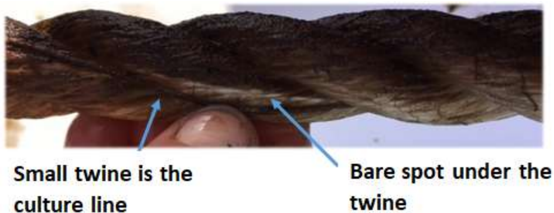
Figure 24: The culture twine is being moved by hand from its original position under tension to reveal a clean section of the long line that was not fouled. This showed that the culture line is secured in place so chafing from excess movement is most likely not the cause of kelp loss.
