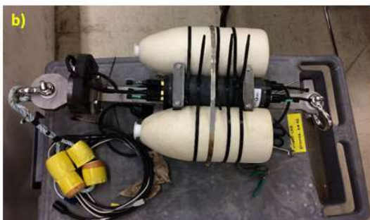
Figure 93: a) Two AWAC instruments will be deployed, one to measure velocity-profiles and the other for measuring directional waves. b) The first load-cell data acquisition system funded by a previous NSF project.
