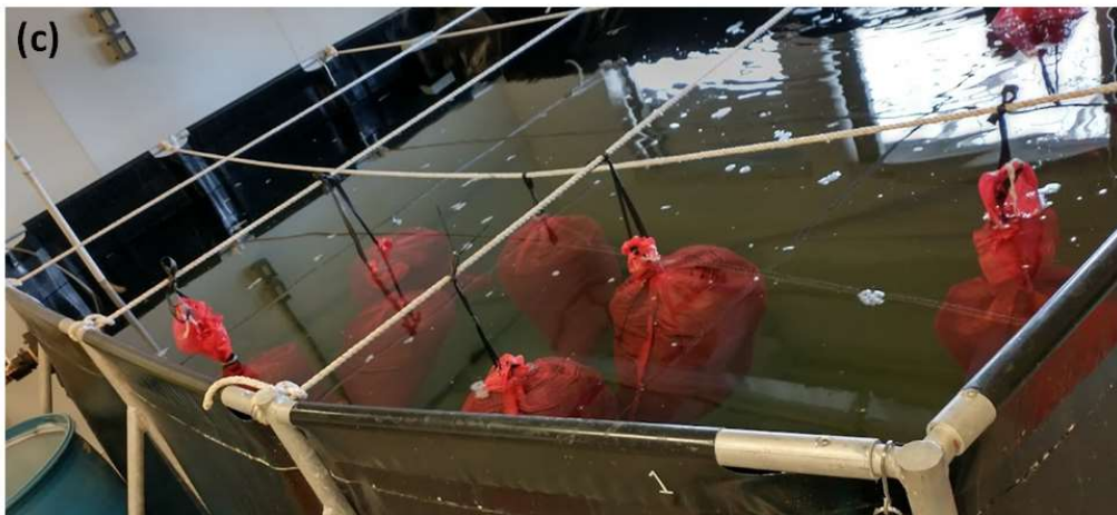
Figure 76: Monitoring of the kelp on 15-April-21 included measuring the length (a), estimating buoy waterline for biomass assessment (b) and performing in/out water weight measurements in still water (c).
