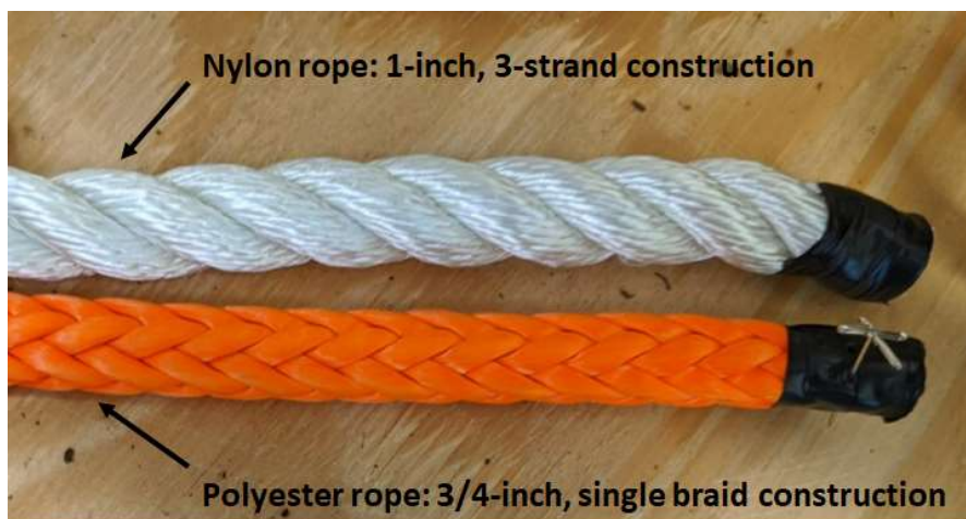
Figure 67: A visual comparison of the nylon grow-line with the polyester (PE12) grow-line to be deployed during the 2020-2021 season.
