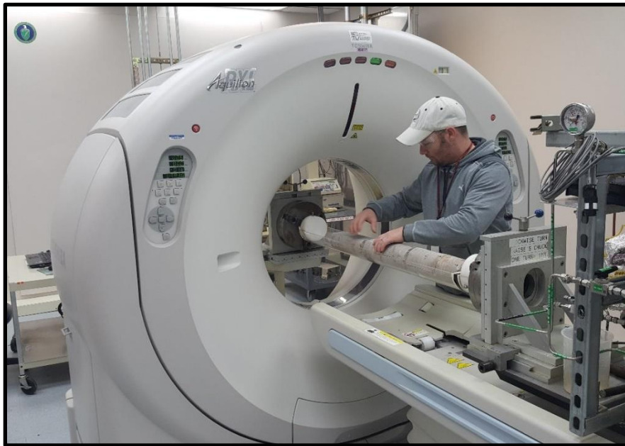
Figure 5: Toshiba® Aquilion™ Multislice Helical CT Scanner at NETL used for core analysis.
