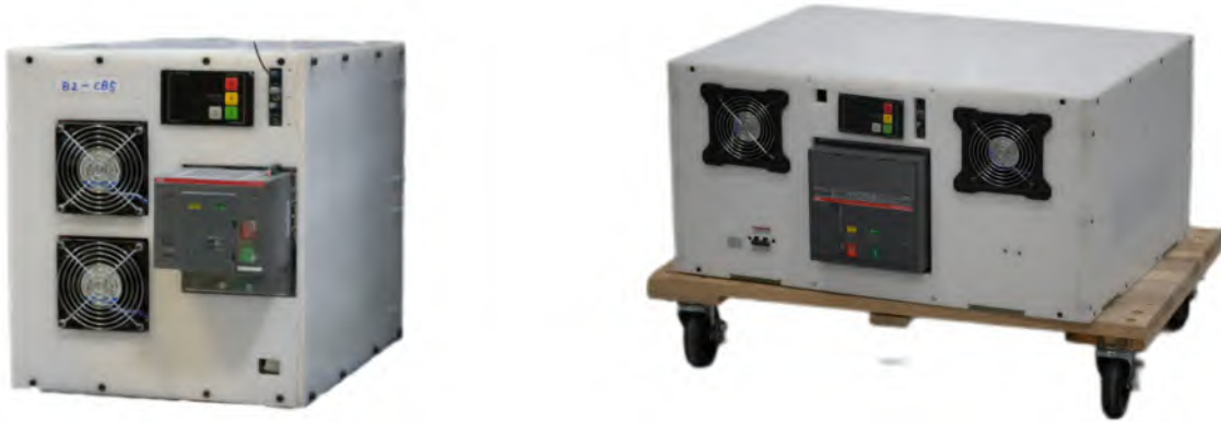
Figure 24: Final version of the 500 A (CB3...6) Class DC SSCBs and 1500 A class DC SSCBs (CB1 and CB2).
