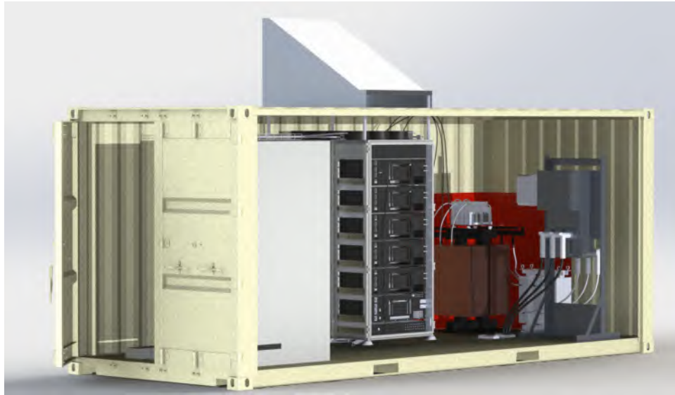
Figure 34: System integration within the shipping container. On the left hand side is the ABB solid state DC circuit breaker. In the middle is the SST. The right hand side is the MV filters.
