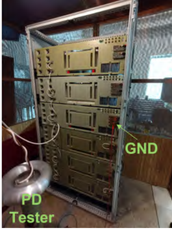
Figure 15: Cabinet level partial discharge test setup
