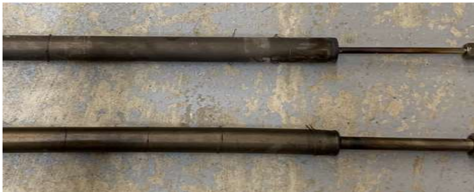
Figure 5.1-35 Upper Section of RFR showing Upper Instrumentation Tubing
