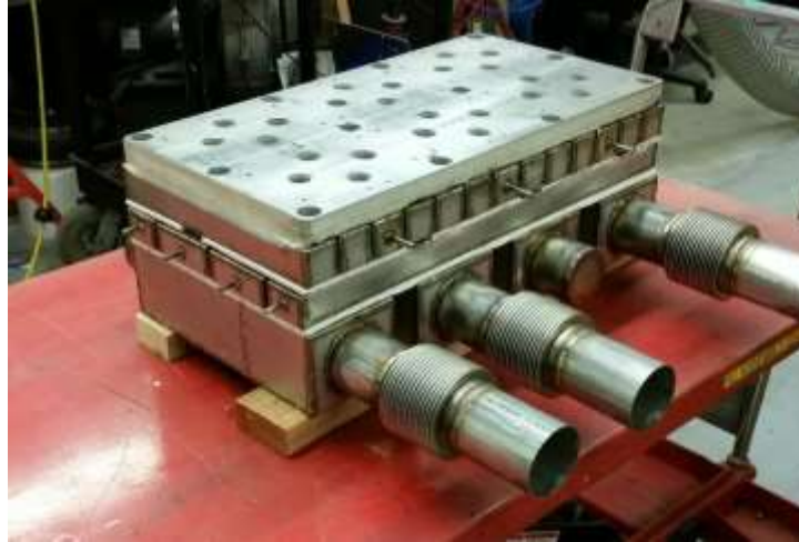
Figure 5.1-57 Stack Distribution Base Assembly (Welded Version)
