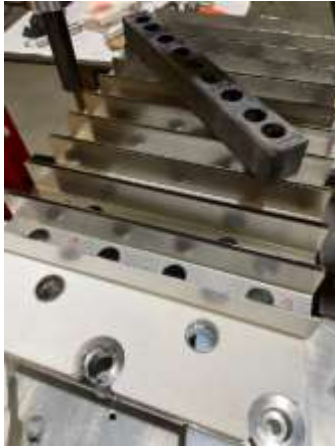
Figure 5.1-37 Stack Distribution Base Brazement Subassembly in Progress
