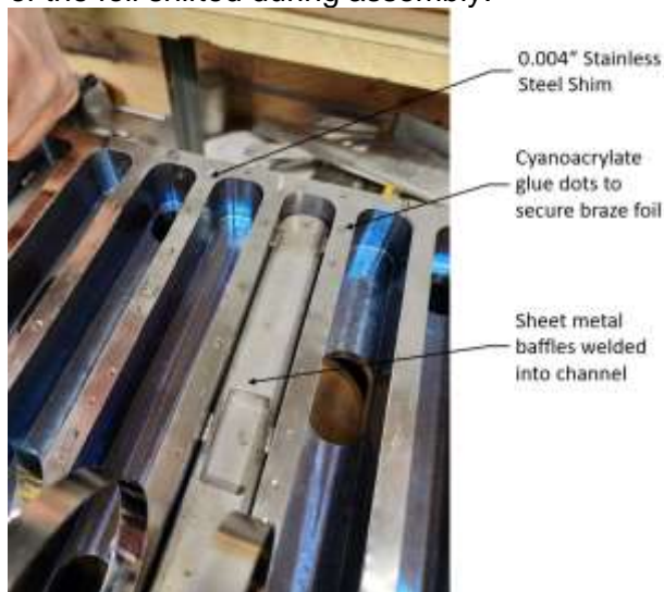
Figure 5.1-60 Assembly Details of Stack Distribution Base
