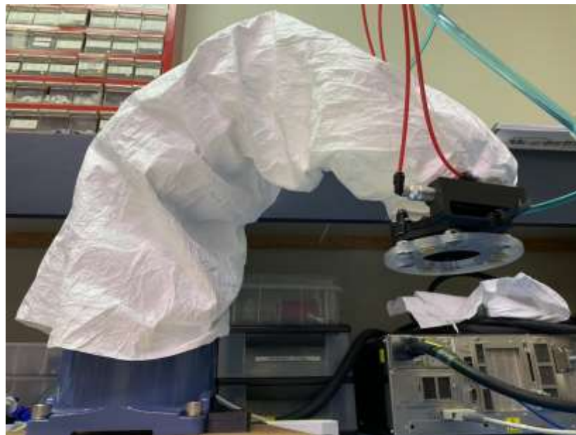
Figure 2.2-4 Cell Grinding Robot with Cell Gripper and Protective Cover
