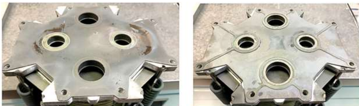
Figure 3.2-20 Original base plate (left) and revised base plate (right)
