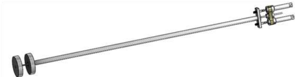
Figure 3.2-11 CAD view of the interface material test jig.
