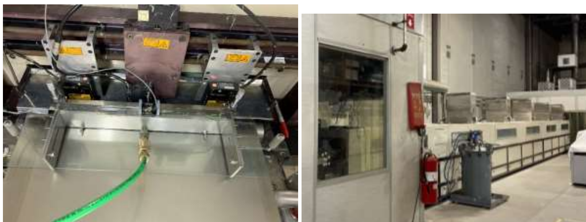
Figure 2.2-9 Revised low-volume level-controlled casting box (right) installed at head of tape caster (right)
