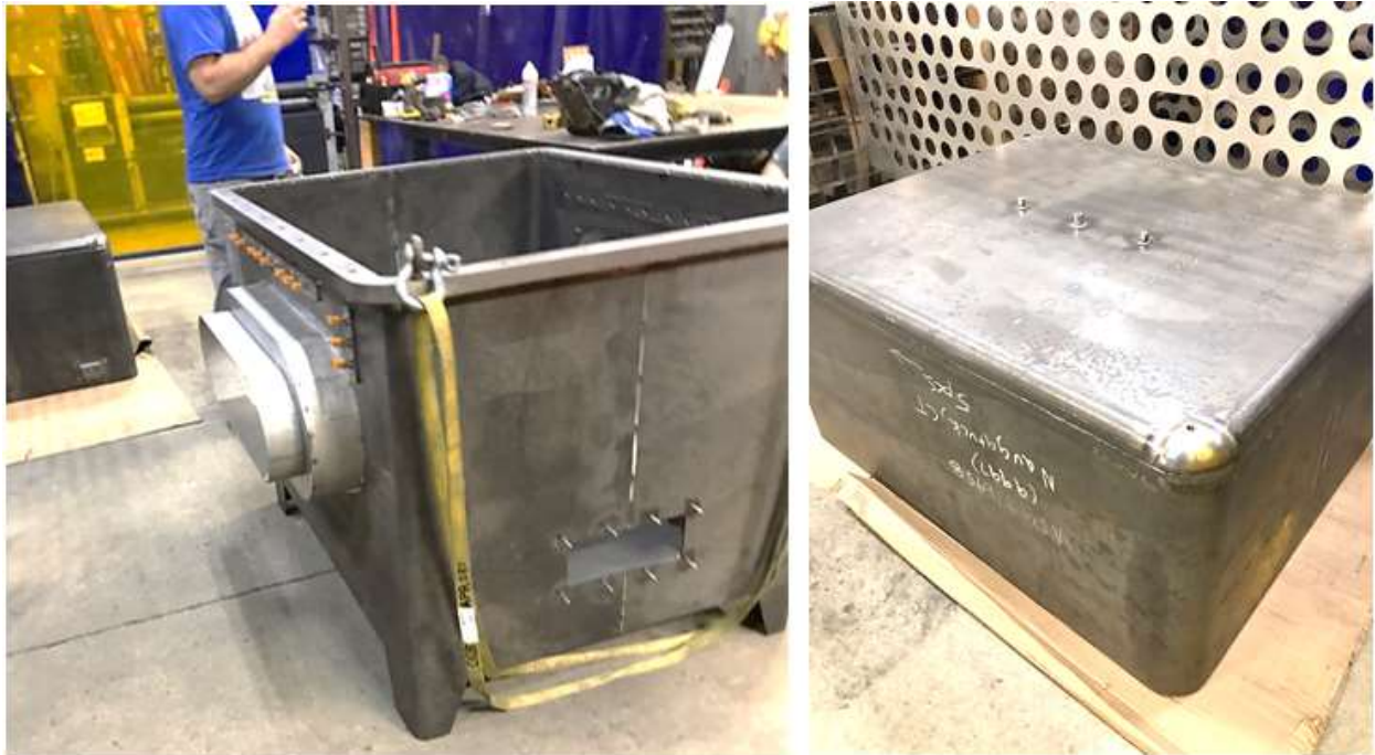
Figure 5.1-13 Fabricated Module Enclosure: Lower Enclosure (left); Upper Enclosure (right)
