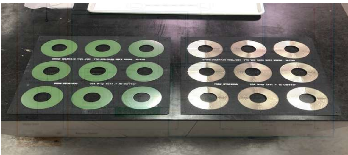
Figure 2.2-8 Parts Pallet-loaded with cells (left) and interconnects (right)
