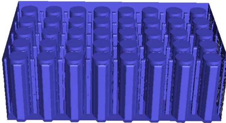
Figure 4.2-16 40-stack module with 280 kWe electrical power.
