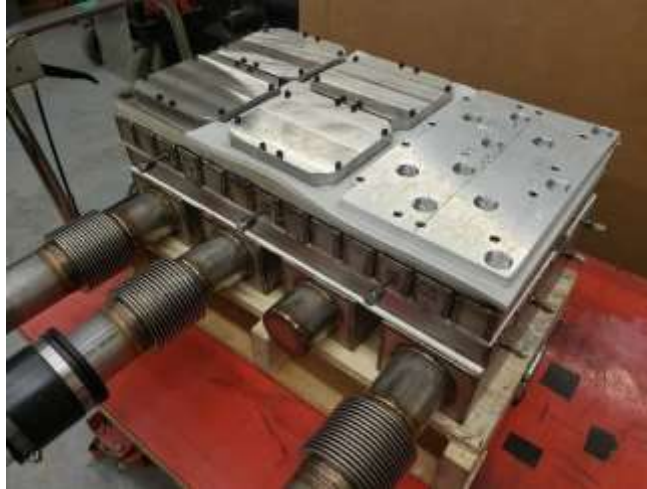
Figure 5.1-40 Top Plate C-ring Seal Leak Test
