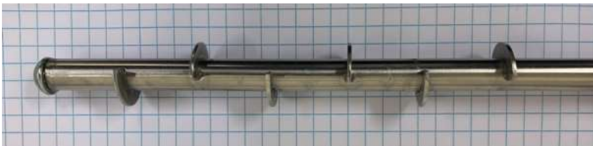
Figure 5.1-56 RFR with Half-Moon Baffles Welded to RFR Lower Portion
