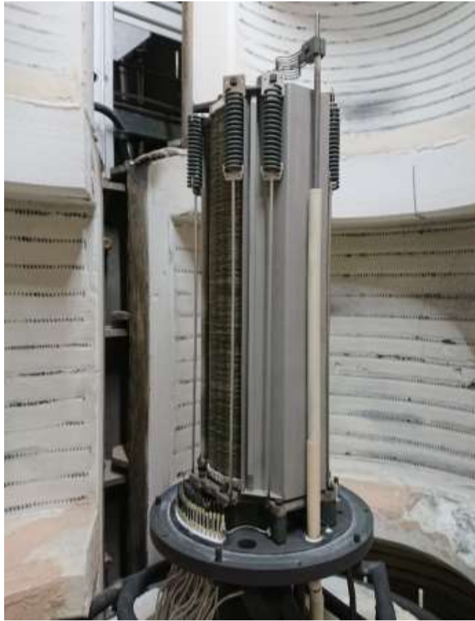
Figure 3.2-7 First Full Height CSA Stack Installed in Test Stand
