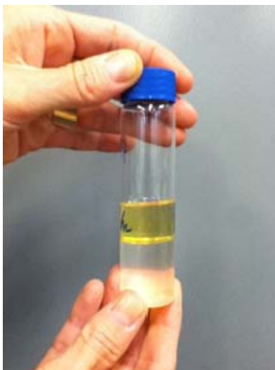
Figure 22. 2-phase liquid product formed by the conversion of 2-butanol over H-ZSM-5(30) catalyst.
