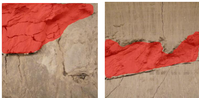
Figure 7-8. Mask R-CNN prediction of borehole wall damage zones (red) on two test images.
