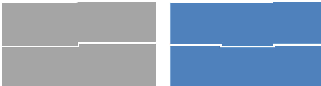
Figure 4.1 Concepts for microchannel geometries with manufactured tortuosity.
