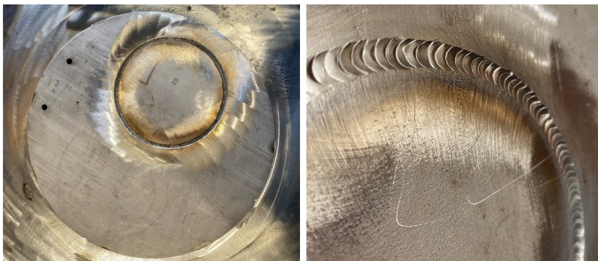
Figure 4.10 SCC plate before (left) and after (right) welding the “outer” side.
