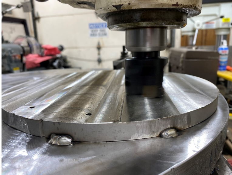
Figure 4.11 End mill was used to plane down the surface of the plate, removing the deformation caused by welding.
