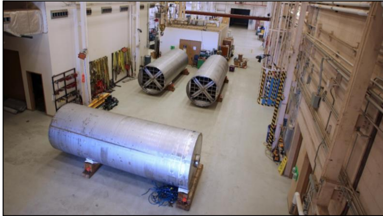
Figure 1.5 Three 32PTH2 spent fuel canisters located inside of SNL's Building 6630 south high bay for preliminary heater testing.
