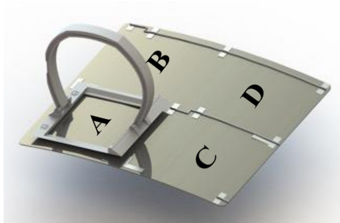
Figure 2.36 Drawing of the mock sampling plate and sampling template used for the simulated field testing.
