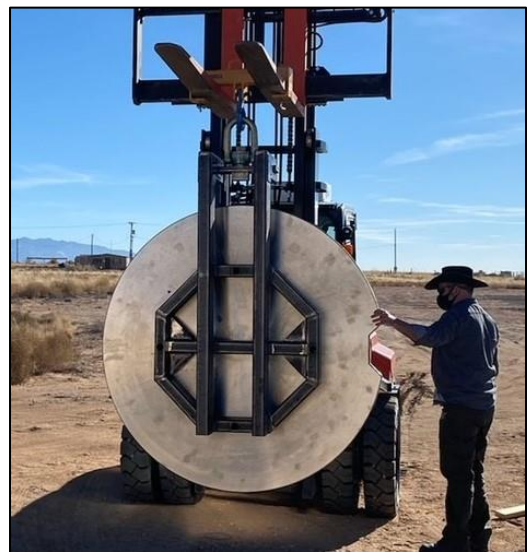
Figure 2.6 Lifting fixture allows OTC to be installed into canister horizontally.
