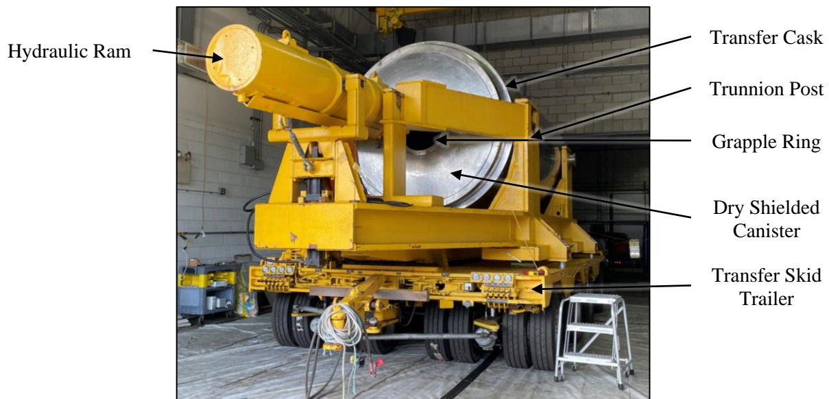
Figure 2.8 Canister transfer skid located at an ISFSI used for inserting dry shielded canisters into storage modules with the use of a hydraulic ram.
