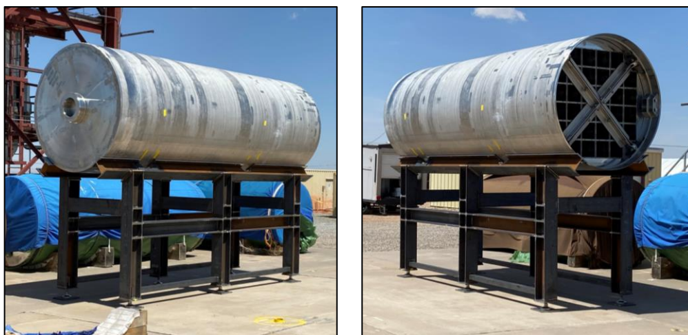
Figure 2.33 32PTH2 dry shielded canister at prototypic height of 8'10" from ground to central axis of the canister.
