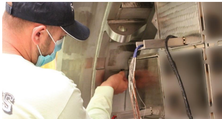
Figure 3.6 Canister-basket gap measurements taken with a wedge gauge at the 300^\circ location on the canister while at ambient temperatures.
