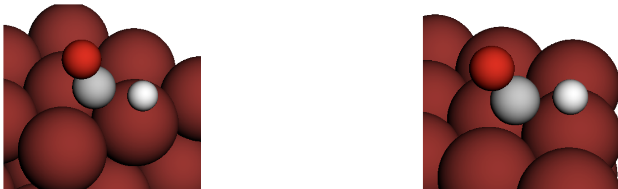
Figure 7: Saddle points for \text{OCH}^* + * \longleftrightarrow \text{OC}^* + \text{H}^* on Cu111. From left to right barriers are: 0.969 eV and 0.979 eV.
