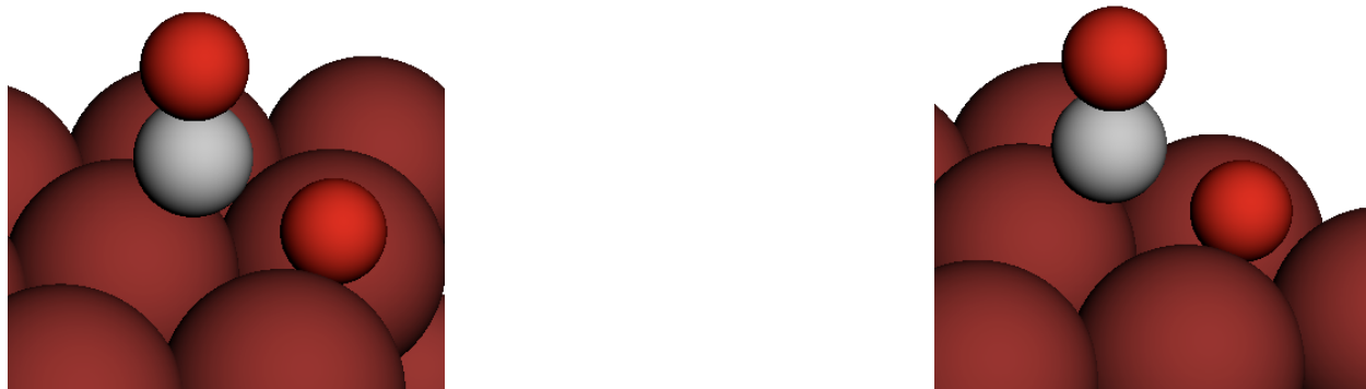
Figure 9: Saddle points for \text{OC}^* + \text{O}^* \longleftrightarrow \text{CO}_2 + 2^* on Cu111. From left to right barriers are: 0.441 eV and 0.441 eV.
