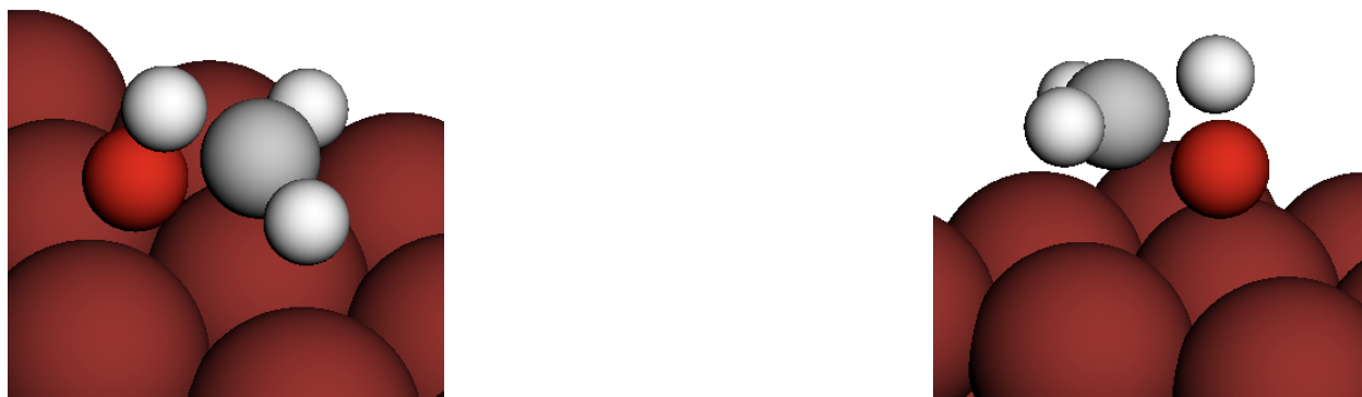
Figure 11: Saddle points for \text{HOCH}_2^* + * \longleftrightarrow \text{CH}_3\text{O}^* + * on Cu111. From left to right barriers are: 2.150 eV and 2.140 eV.
