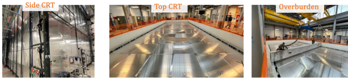
Figure 6. From the left: the sides CRT modules, the Top and the installation of the overburden's concrete blocks (eventually a 3 m thick layer).
