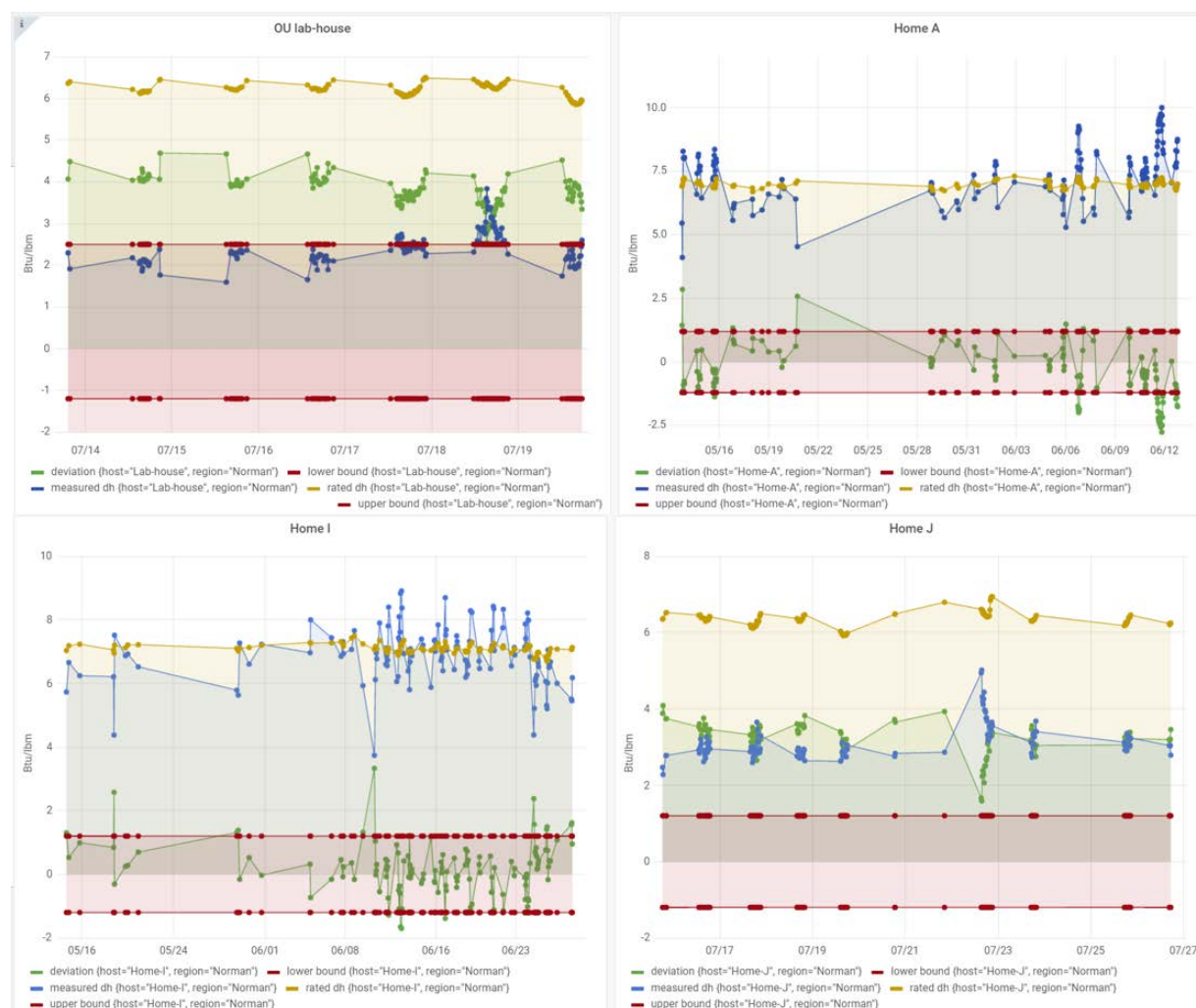
Figure 7.11. Real-time monitoring of enthalpy change across the evaporator for four test homes for Phase 1
