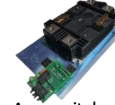
Aux switch w/ gate drive 4.5 kV 60 A Si IXBX50N360HV
