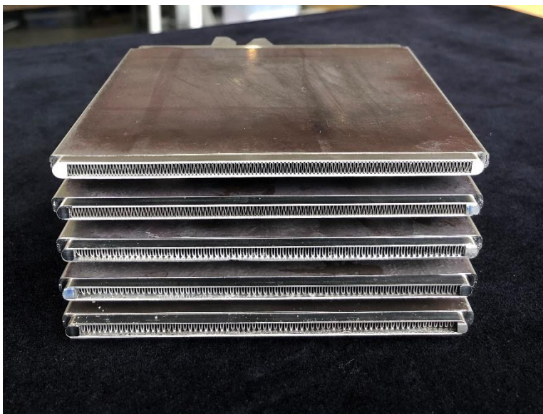
Figure 16: Folded fin test article figures (top) drawing detail (center) flat-crest fin (bottom) round crest fin
