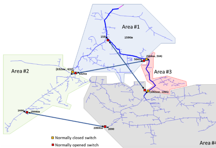
Figure 55: Diagram of 2500 nodes distribution system with inter-area switches
