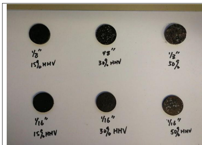
Exhibit 6. Typical plastic/biomass blend pellets prepared with the Buehler Pelletizer, in the form of plastic energy input to blend fuels.
