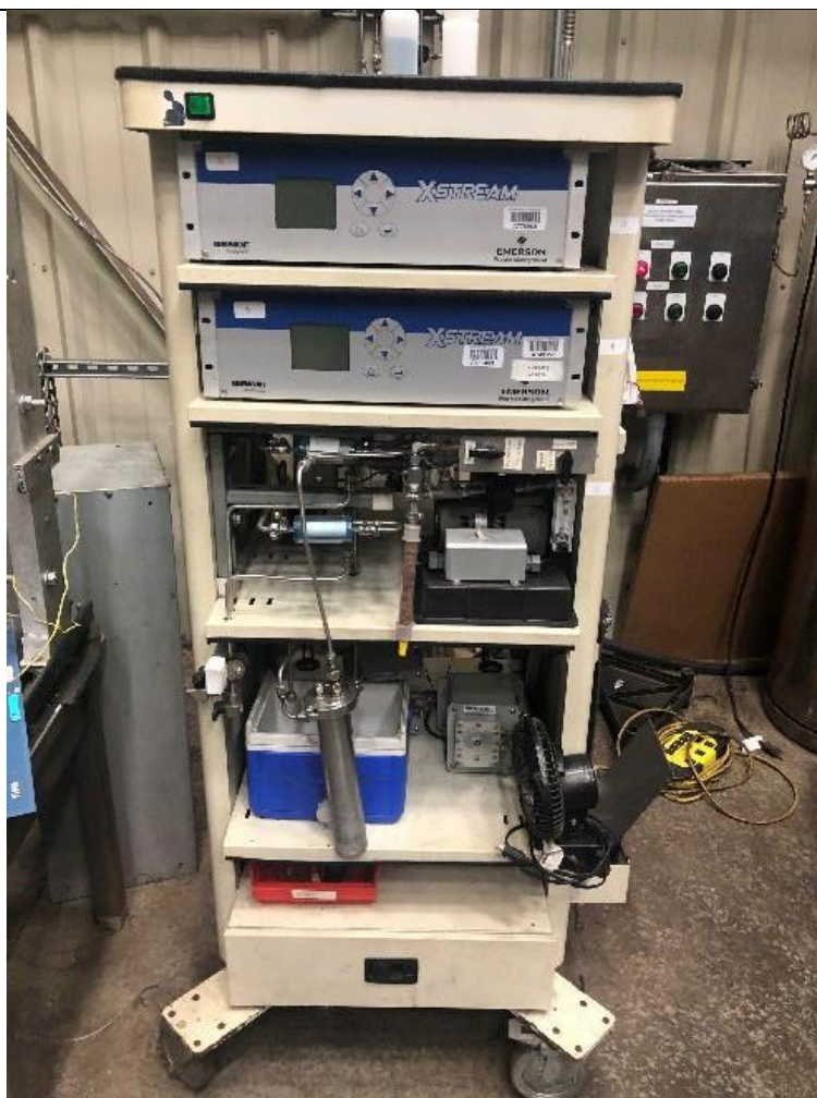
Exhibit 59. X-stream Gas Analyzer System including Two Analyzers, Vacuum Pump, Condensation Trap, and Silica Beads.
