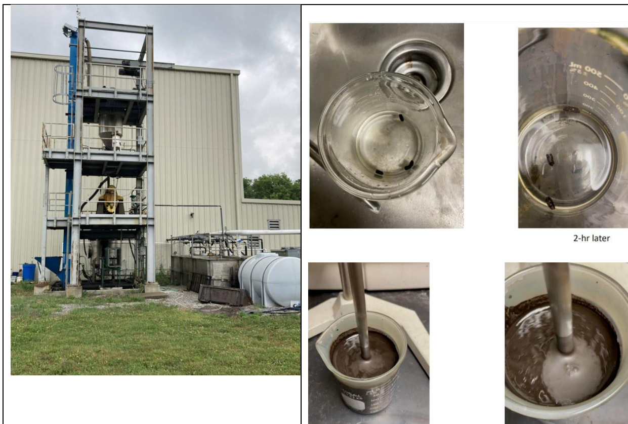
Exhibit 68. UK 4-Level Slurry Preparation Unit (Ball Mill, Weight Belt, Coal Hopper) was Operated (Left). The water intake of the produced pellets was tested for 2 hrs (upper right). Two slurries of coal/biomass-plastic blend 55 wt% and 50 wt% were produced (bottom right).
