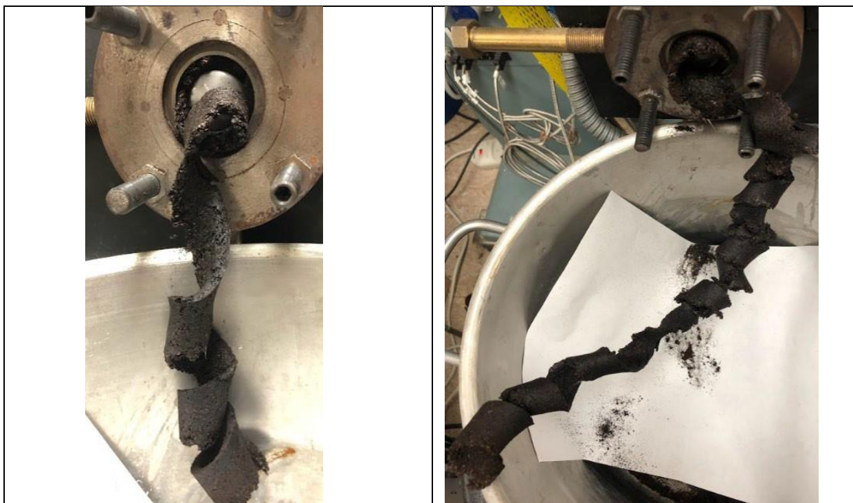
Exhibit 18. Extruder Testing Result (without die) with Mass Ratio of HDPE:TW = 1:1
