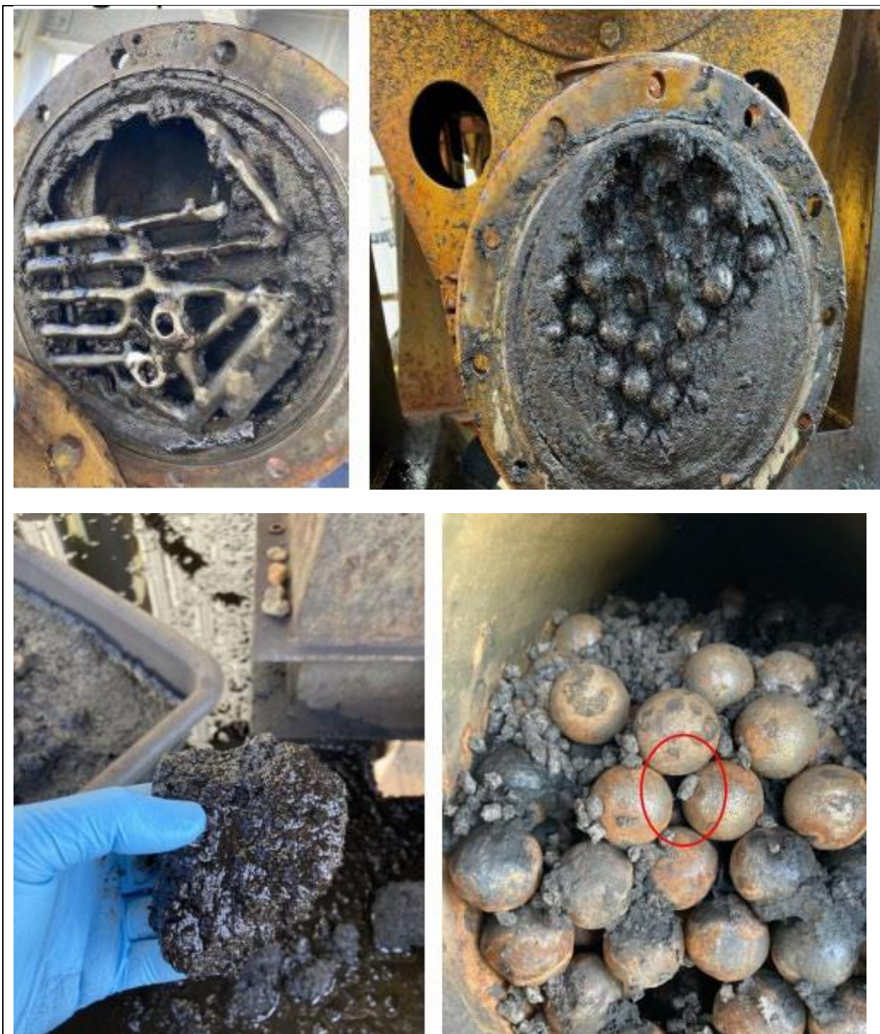
Exhibit 69. During Operation of the Ball Mill the Outlet Screen Broke (Top). The lower section, on the other hand, had mostly coal slurry, and the presence of biomass may have absorbed most of the water, resulting in a thick paste-like slurry (bottom).
