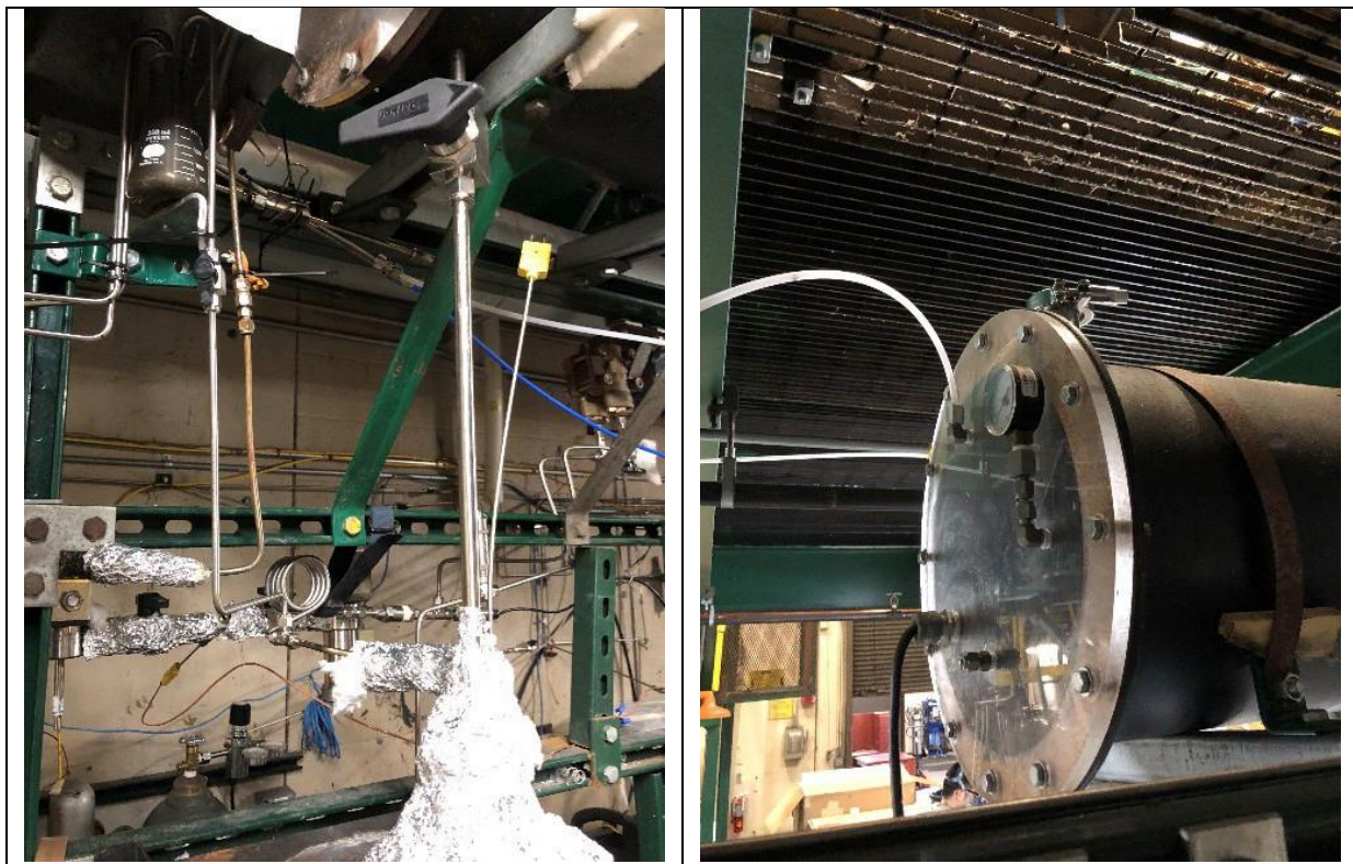
Exhibit 60. Modified Reactor Setup with a Dedicated Solid Inlet (left). Nitrogen Line Connected to the Vibration Feeder with a Quick Connection Cap to Pressurize the Container (right).
