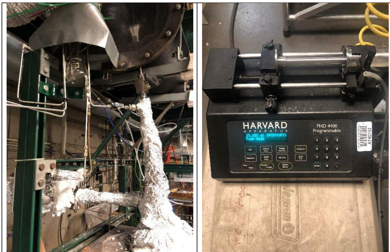
Exhibit 58. Initial Setup of the Reactor. Solid inlet and gas exhaust share the opening into the reactor. The flask located under the fume hood pump captures gas from the reactor or from the mass flow controllers directly for gas analyzer calibration. The input of the gas analyzer is in the flask situated above the others (left). Harvard Apparatus PHD 4400 water pump (right).
