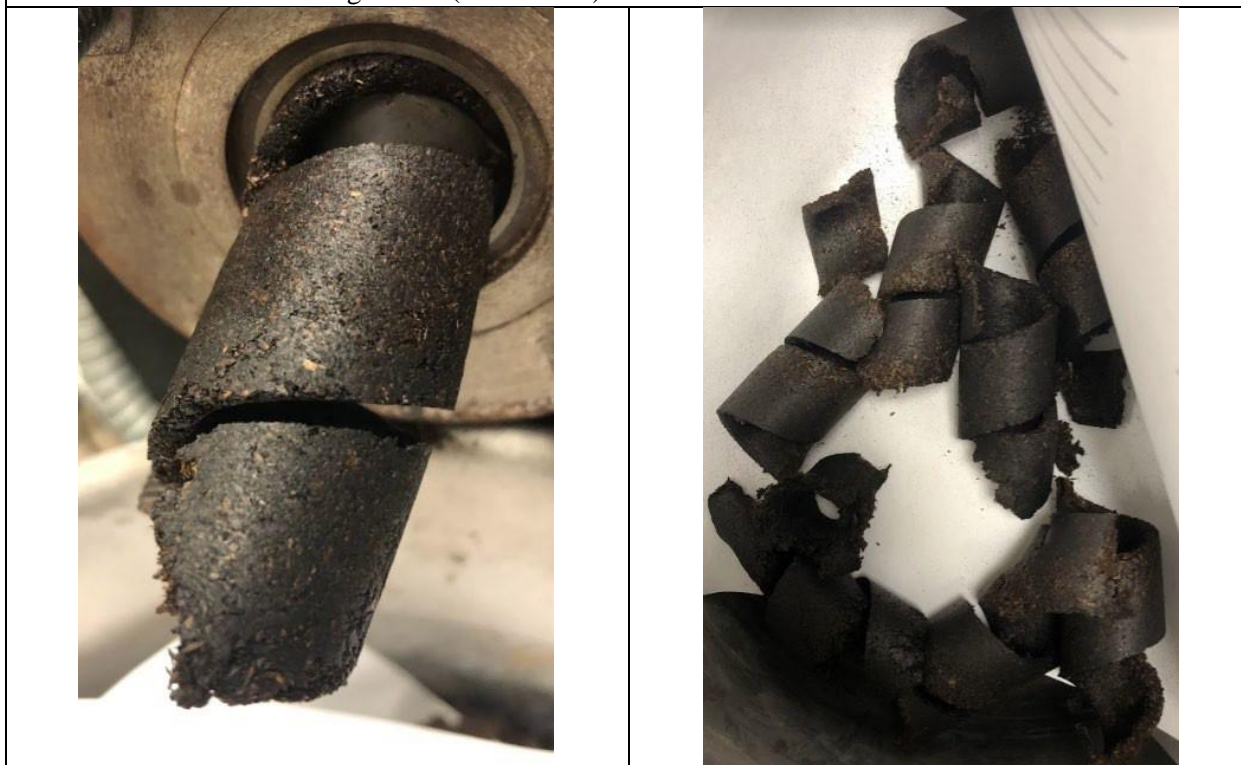
Exhibit 19. Extruder Testing Result (without die) with Mass Ratio of HDPE:TW = 1:2
