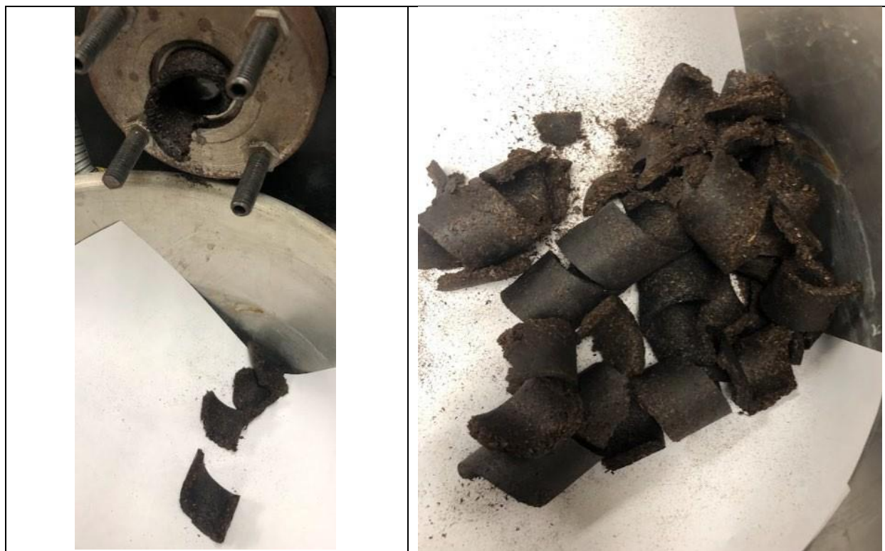
Exhibit 20. Extruder Testing Result (without die) with Mass Ratio of HDPE:TW = 1:4
