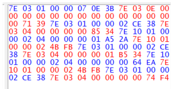
Figure 4.53 – Communication between the XCTU software and the embedded Modbus RTU module via a USB connection, the blue bytes in hexadecimal represent the manually input command request while the red bytes are the response from the FPGA
